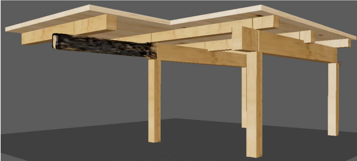
Figure 25: Illustration of building Cross-Section with Charred Girder
