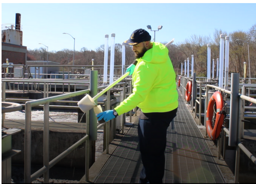
Figure 5: Wastewater Treatment Operator Collecting Treatment Sample for Testing (Fairhaven Water Pollution Control Facility, 2022)
