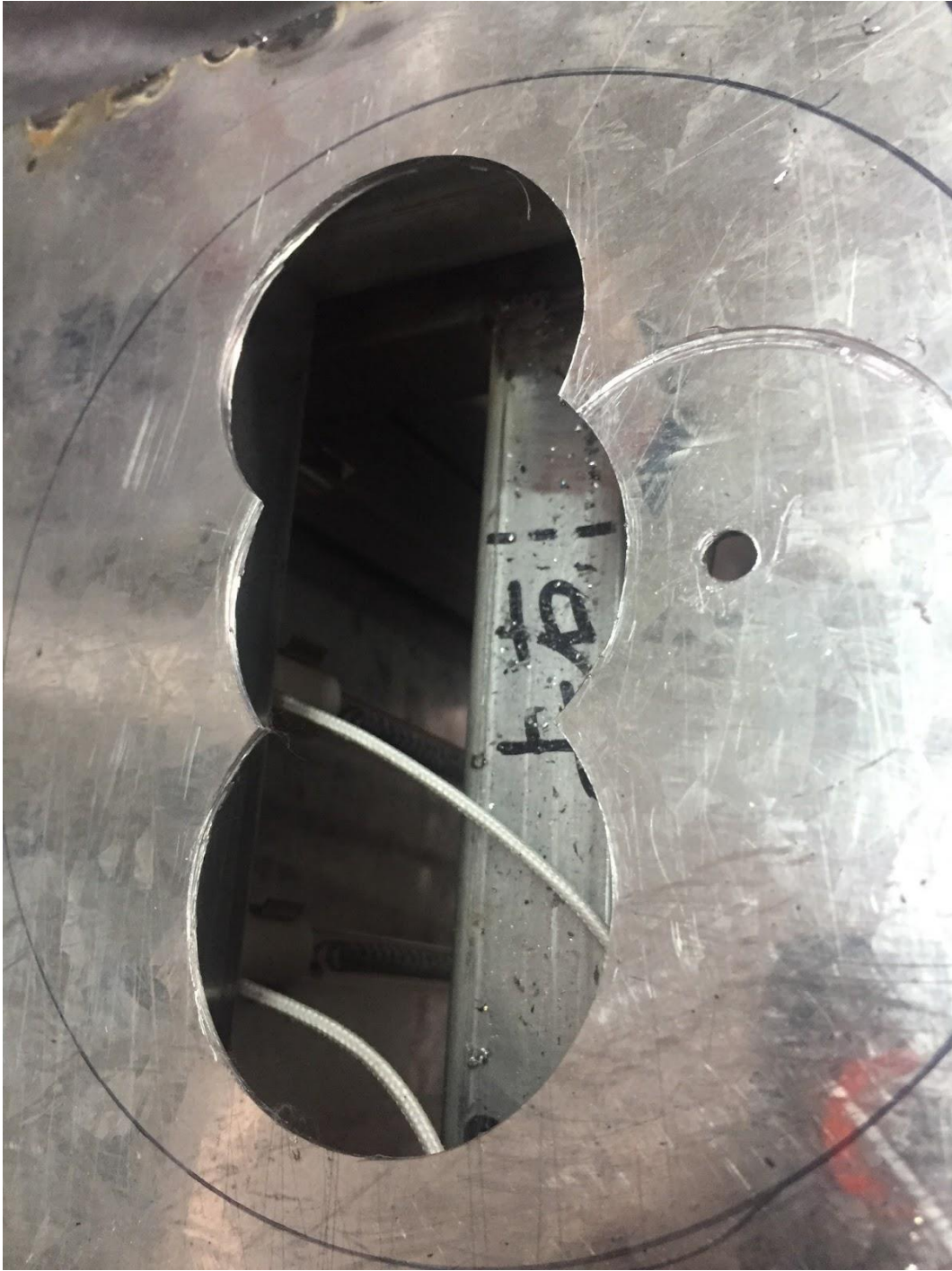
Figure 24: Drilling the Hole for the Fan
