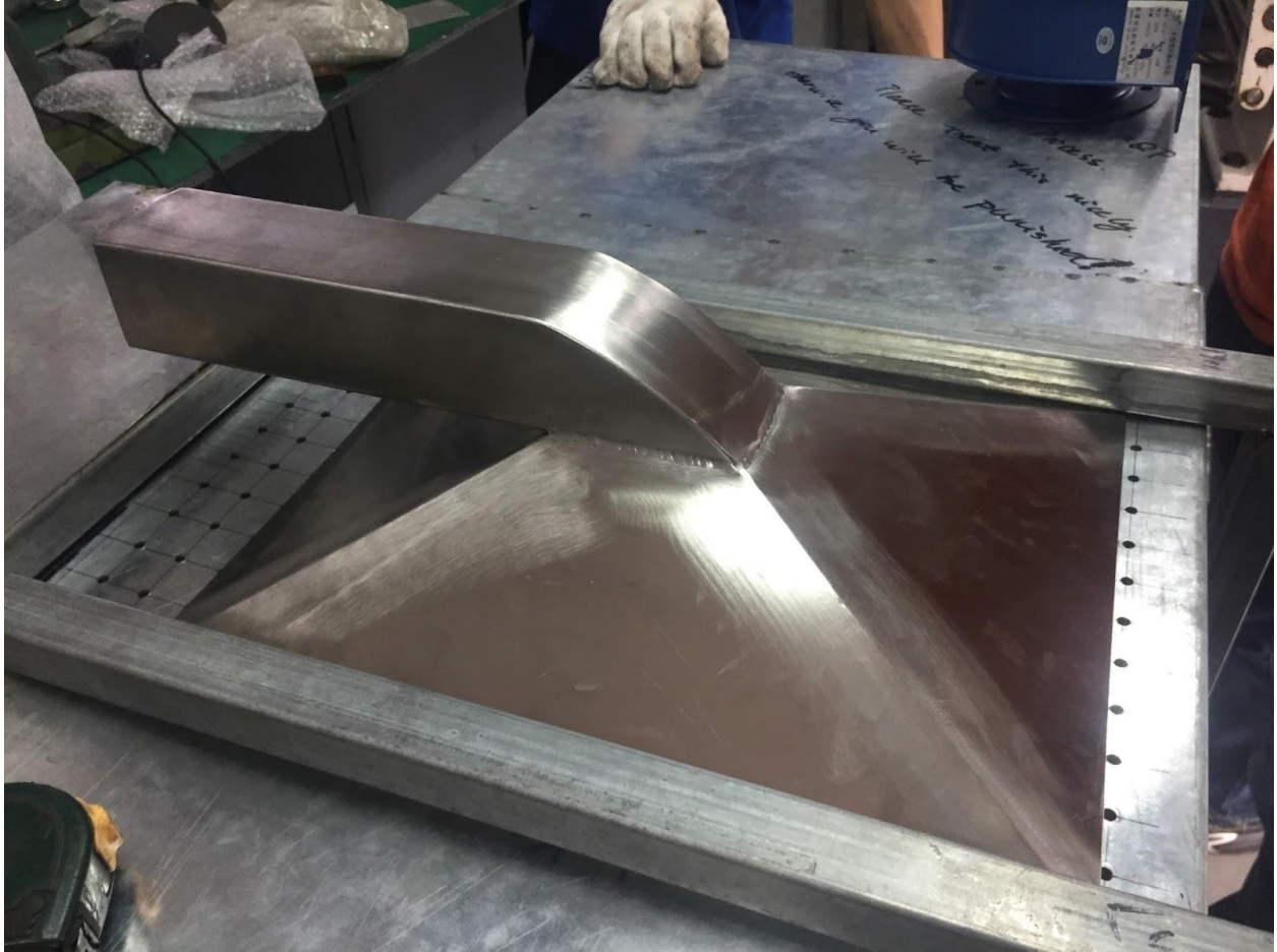
Figure 23: Vent for the Drying Oven Prototype
