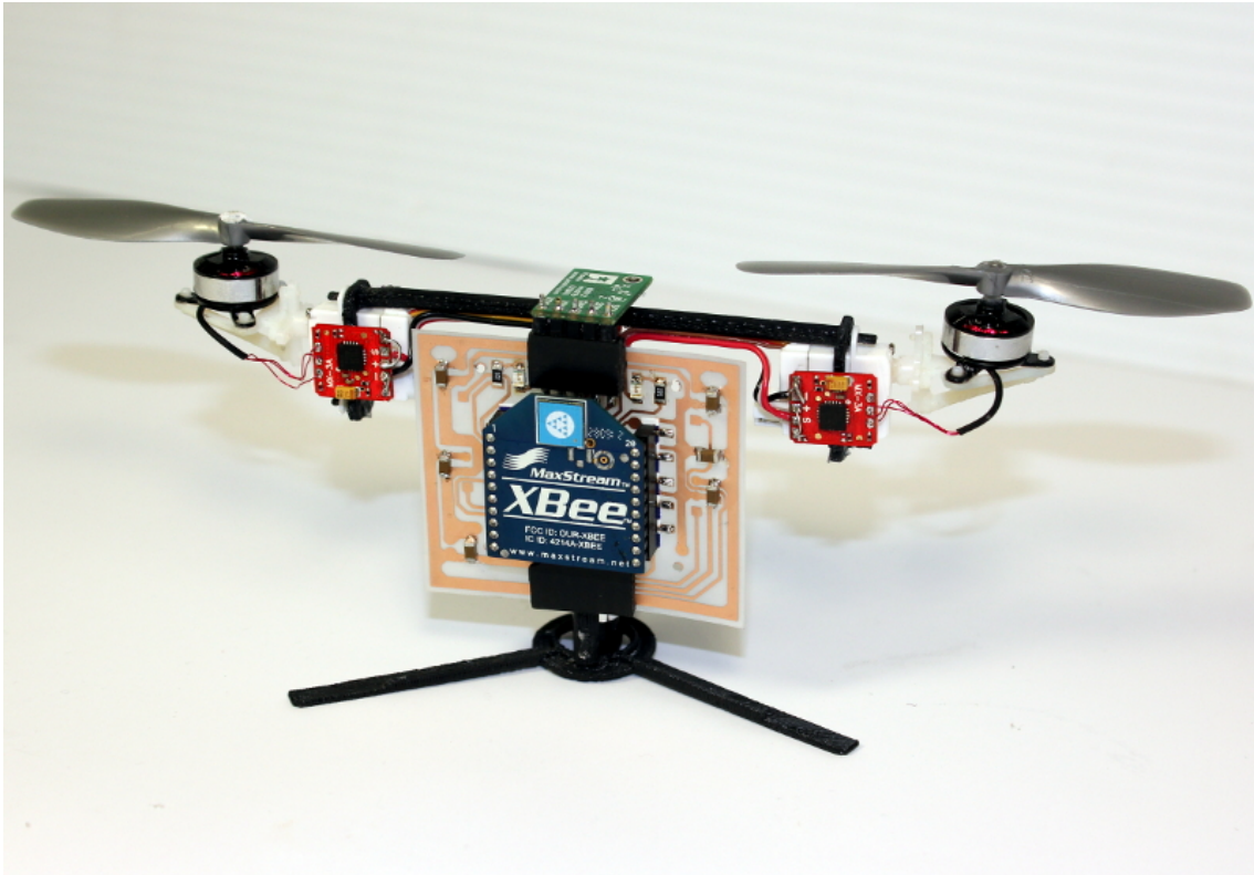
Figure 4.14: The realized micro scale tiltrotor.
