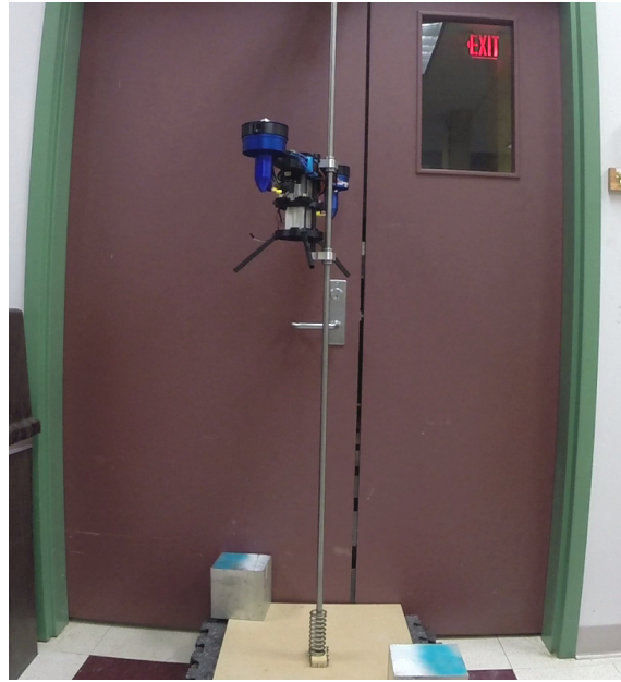
Figure 5.11: TRo hovering with remotely controlled altitude and yaw control.
