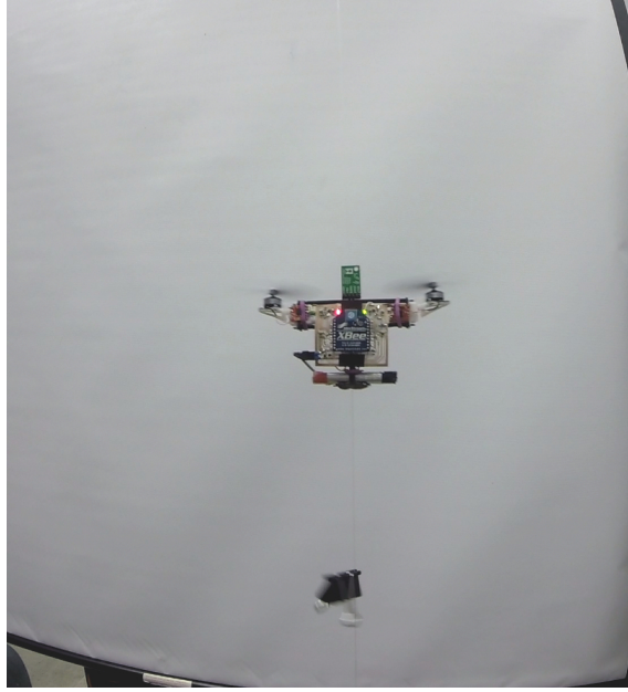
Figure 5.10: \mu TRo hovering with remotely controlled altitude and yaw control.
