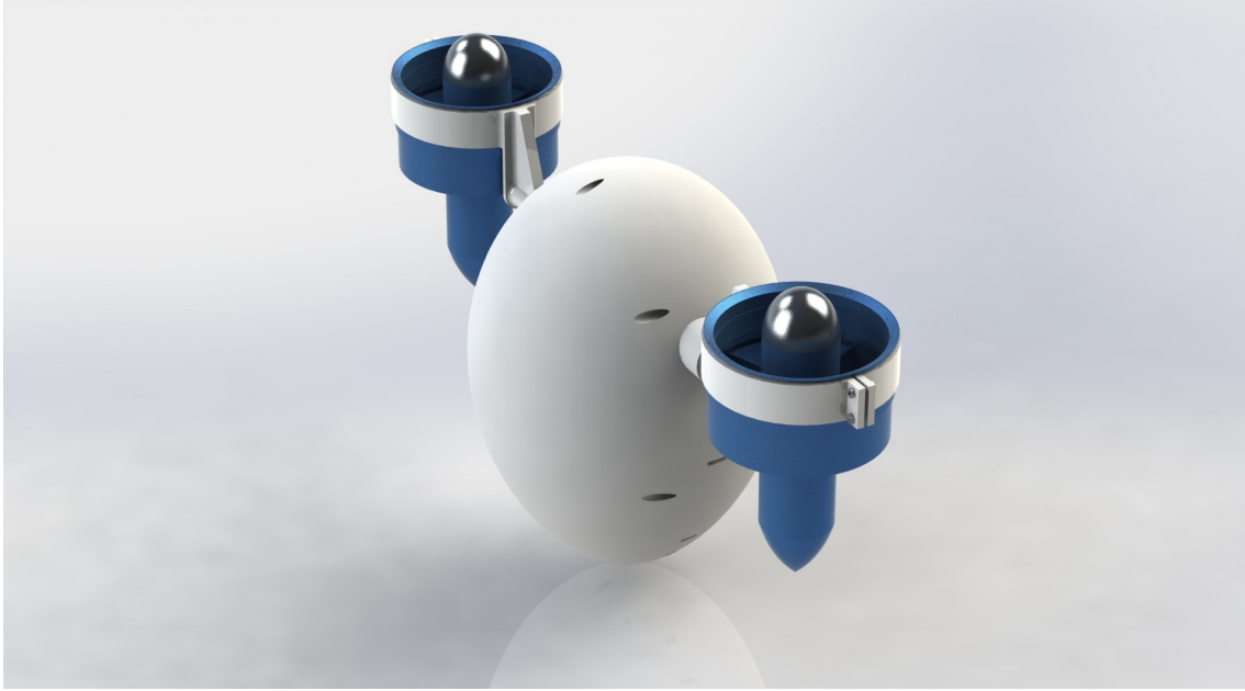
Figure 1.2: The proposed dual-nacelle tiltrotor concept aerial vehicle
