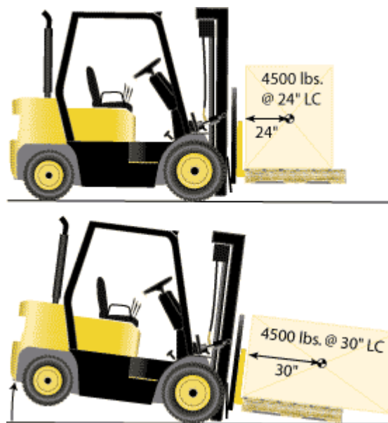
Figure 7: OSHA Forklift Tipping Demonstration
