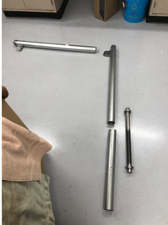
Image 6: Cut Galvanized Posts and Filed Steel Rod
