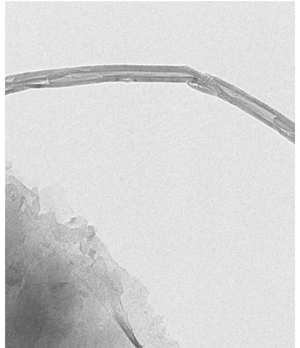
**Figure 13** TEM images of multi-walled carbon nanotubes grown on iron deposited on silica/Si wafer with propylene as carbon source. The diameter varied between 30 – 60 nm. Walls of the nanotubes do not show uniformity of structure showing many defects.
