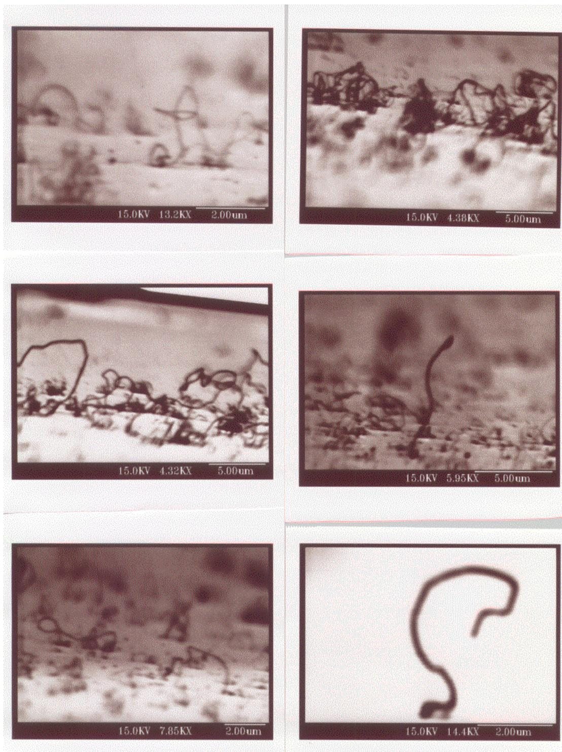
**Figure 7** SEM scan of sample reacted at 900 °C at reduced benzene to hydrogen ratio shows ample amount of carbon nanotubes formed. Helium flow rate through saturator was 87.3 ml/min
