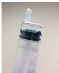
Figure 52 Bead solution sitting stagnant for too long will cause the beads to sink and stick to the plastic syringe.
