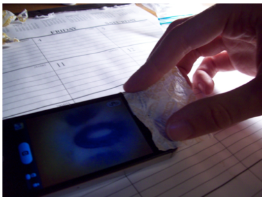
Figure 36 a) Preliminary testing results of imaging writing on paper with 100x magnification b) The resulting image from the iPhone of this imaging test.
