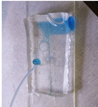
Figure 51 Example of leaking device due to poor bonding
