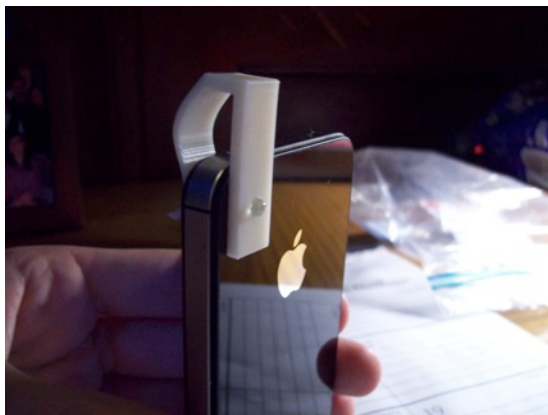
Figure 35 a) 3D-printed plastic clip with bead affixed to iPhone 4S. The bead protrudes from the clip because the hole was printed slightly smaller than it should have been. b) close up image of the microscope bead clip
