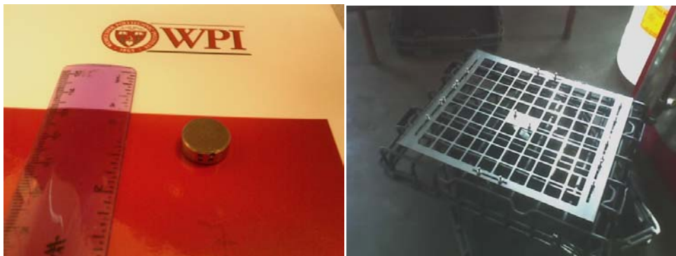
Figure 2 Sample shape and workload used for the nitriding experiments
