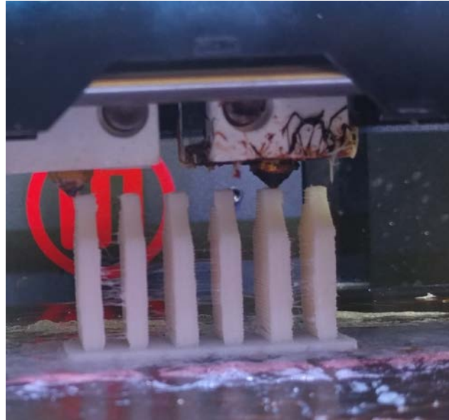
Figure 15: The left nozzle of the MakerBot hitting the leftmost tensile samples, prior to rotating all MakerBot prints 90 degrees on the y-axis.
