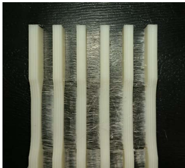
Figure 18: Zortrax 11123 print condition showing severe spider-webbing between tensile samples.
