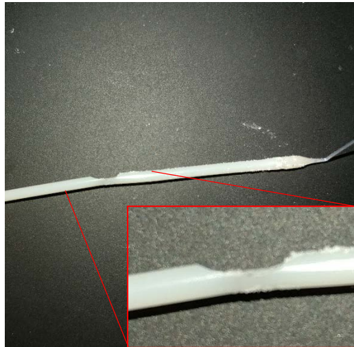
Figure 14: Divot that occurred due to overheating the filament feeder of the MakerBot.
