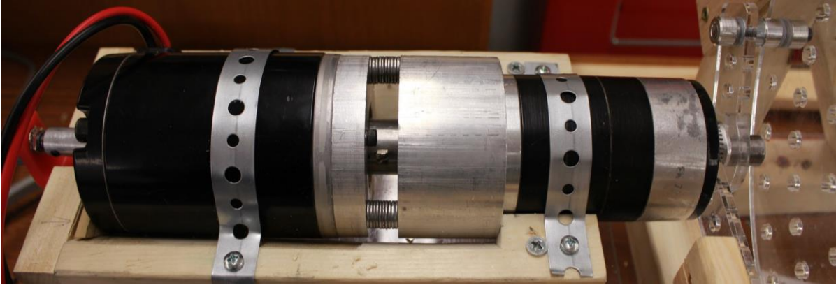
FIGURE 9 PHOTOGRAPH OF DRIVE TRAIN SYSTEM WITH AMP FLOW E30-150 MOTOR AND 52:1 GEARBOX
