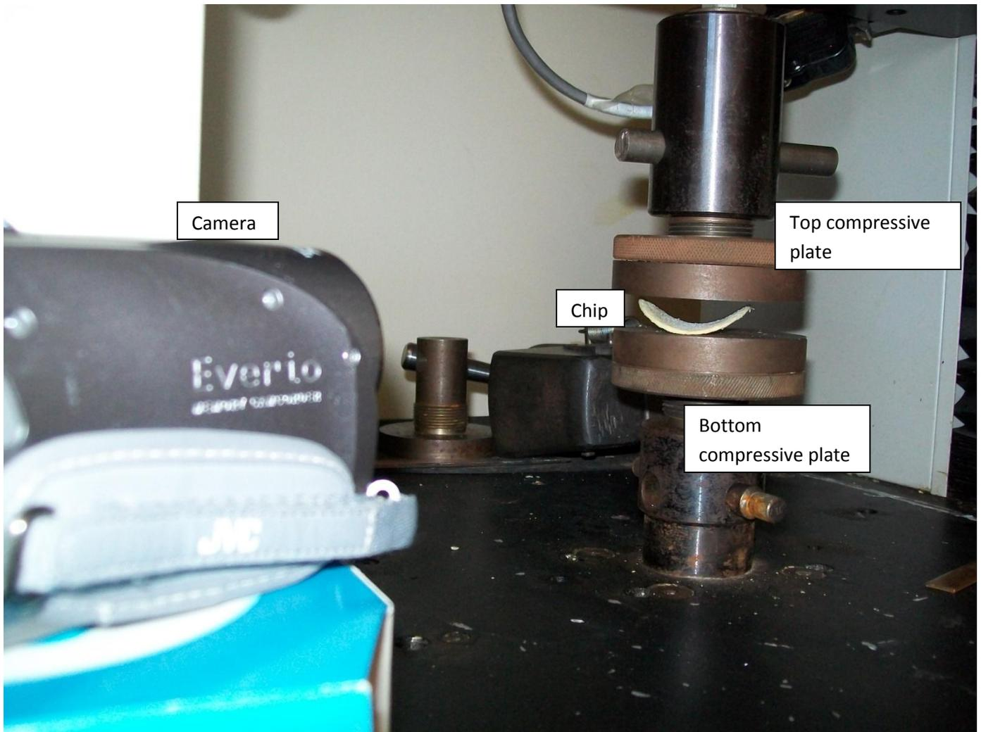
*Figure 4 Compression test set up. The camera was placed on a platform for a better shot of the samples breaking.*
