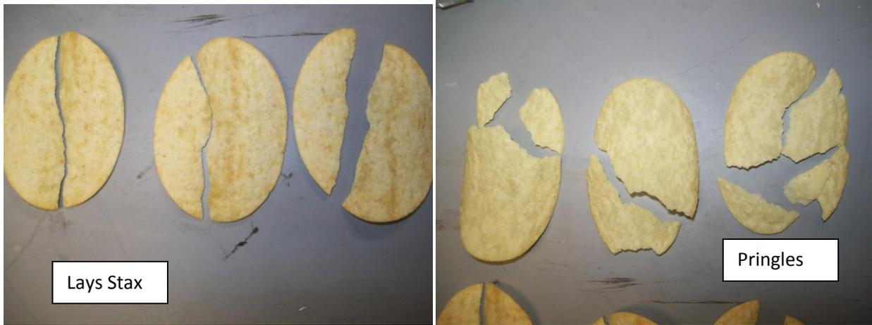
Figure 12 Examples of broken Lays (Left) and Pringles (Right). Lays chips were likely to break down the center flat part of the chip. Pringles would break in a more random pattern.
