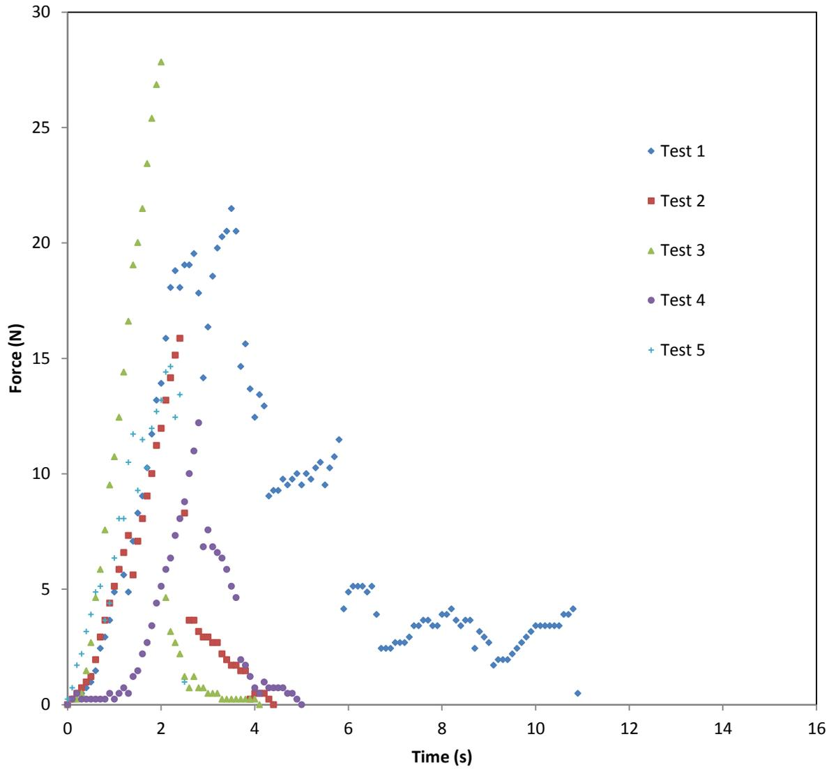
Figure 10 Force verse time graph for the five 3 point flexural test for Stacy's Pita chips.
