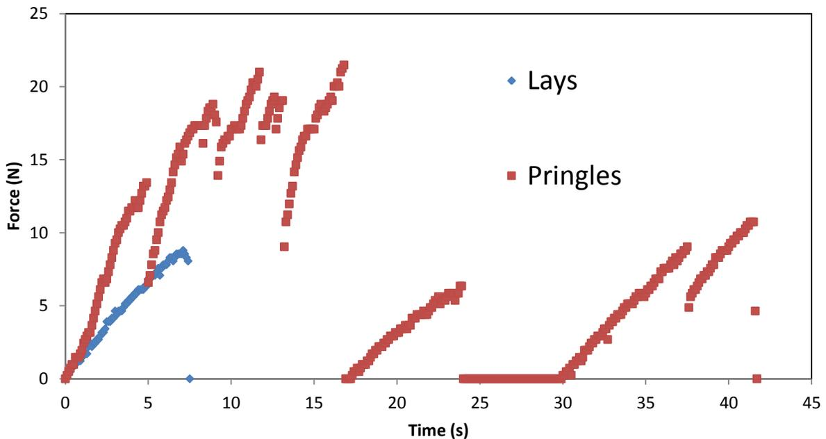
Figure 1 A comparison of the force versus time graphs right when the chips were taken out of packaging. This clearly shows the difference in maximum force, modulus, and number of breaks.
