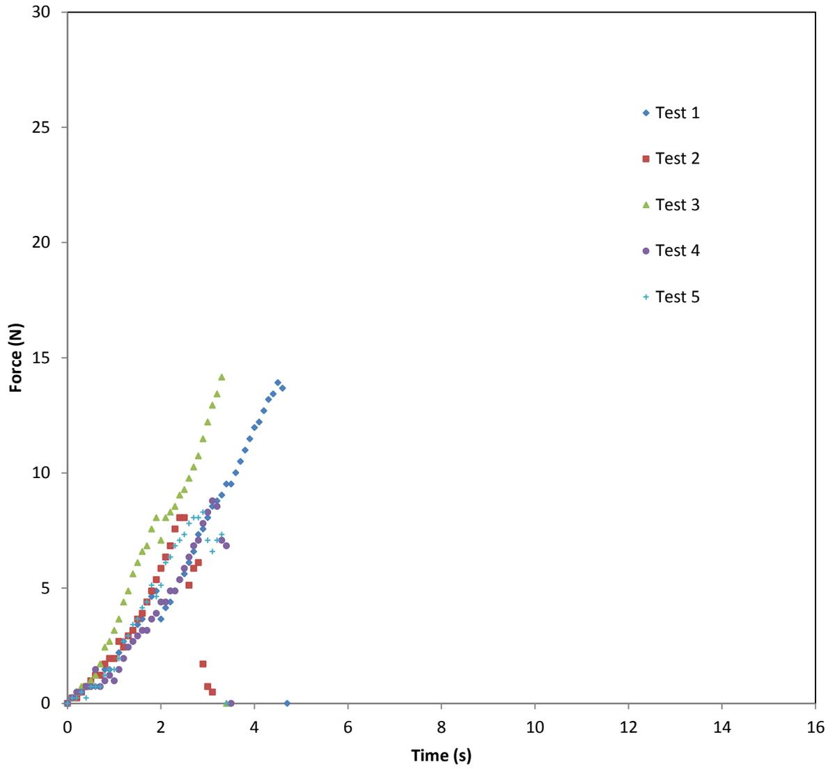
*Figure 8 Force verse time graph for the five 3 point flexural test for Doritos chips.*
