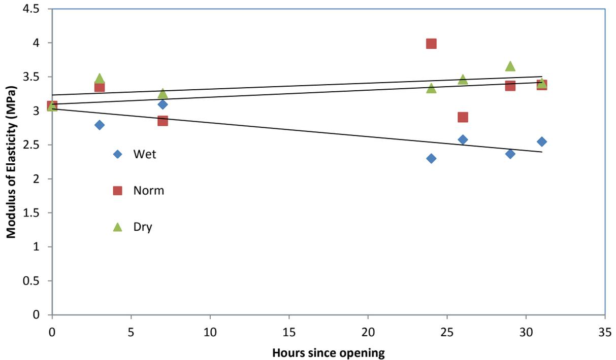
Figure 153 Changing modulus over time for Pringles chips. Samples in wet environment experienced more degrading over time.
