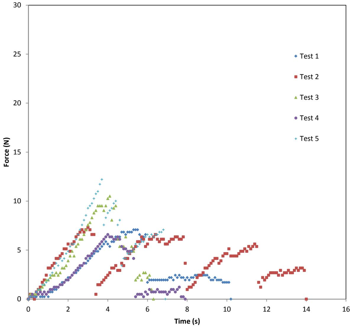
Figure 5 Force versus time graph for the five 3 point flexural test for Lays Kettle chips.
