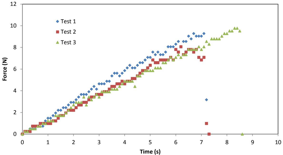
*Figure 11 Three compressive tests of Lays Stax conducted after 29hrs in the dry environment. The similarity of each tests shows that our test was reproducible.*
