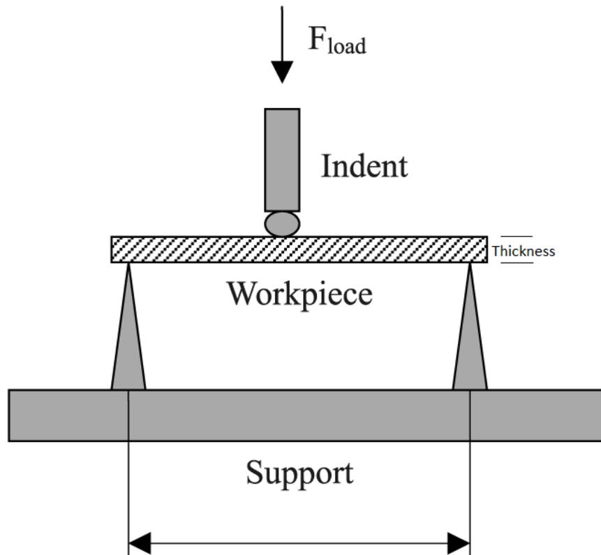
*Figure 3 Set up of three point flexural test showing how thickness and distance between supports are measured.*
