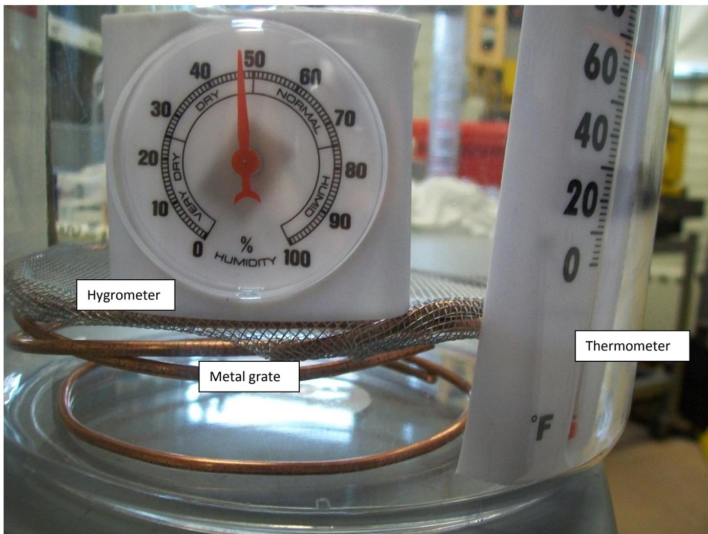
*Figure 5 Sealable container with metal grating to hold the chip up. A thermometer and hygrometer were included to track the temperature and humidity in each container.*
