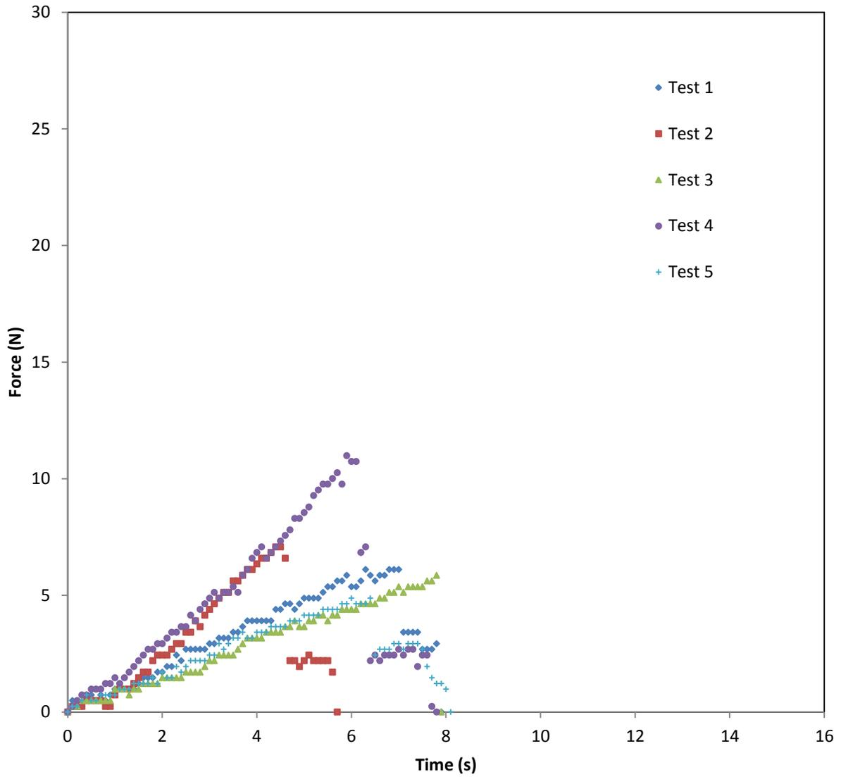
Figure 11 Force verse time graph for the five 3 point flexural test for Ruffles chips.
