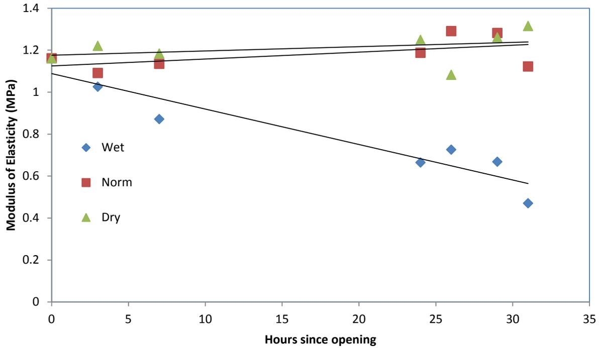
Figure 2 Changing modulus over time for Lays Stax chips. Samples in wet environment experienced more degradation over time.
