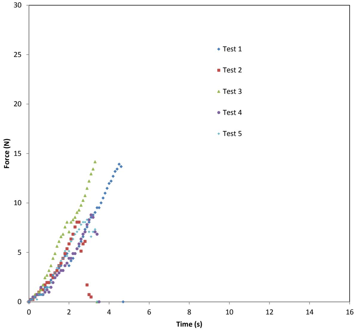
Figure 7 Force versus time graph for the five 3 point flexural test for Fritos chips.
