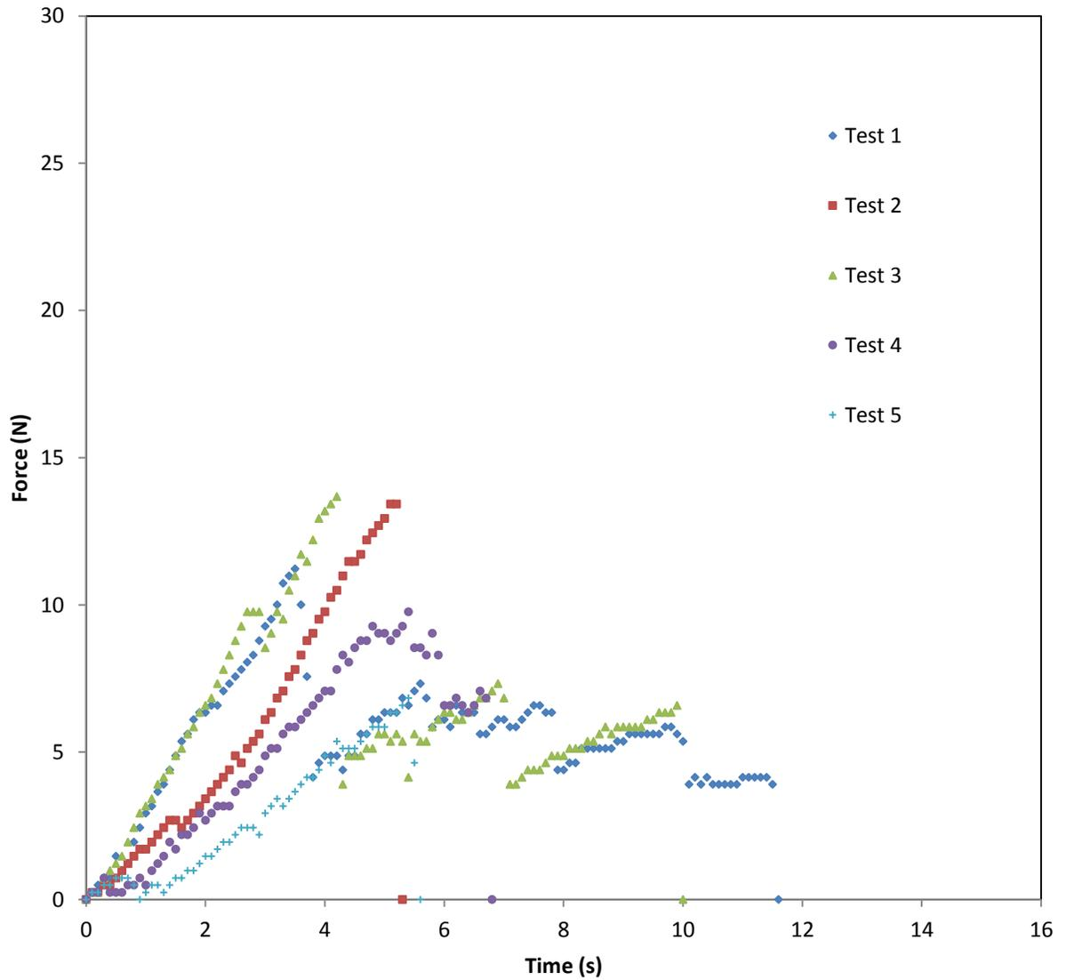
Figure 4 Force verse time graph for the five 3 point flexural test for Cape Cod Kettle chips.
