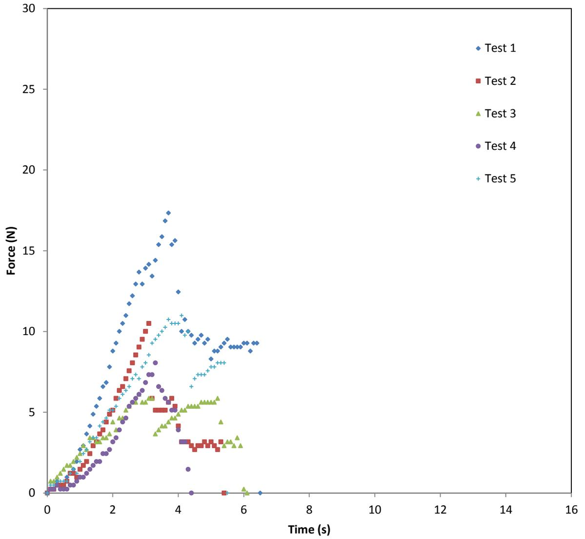
Figure 6 Force verse time graph for the five 3 point flexural test for Price Chopper Kettle chips.
