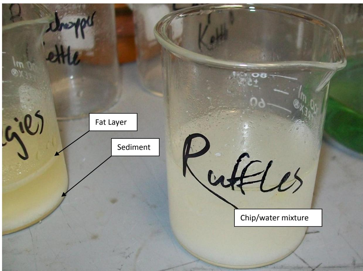
Figure 8 Example of chip/water mixture prior to pH measurement by portable probe. To the right is one rippled potato chip sample (Ruffles); notice the subtle white sediment at the bottom. Clearer separation can be seen in the cut-off beaker to the left, with a fat layer on top, an aqueous heterogeneous chip mixture in the middle, and a sedimentation layer at the bottom.
