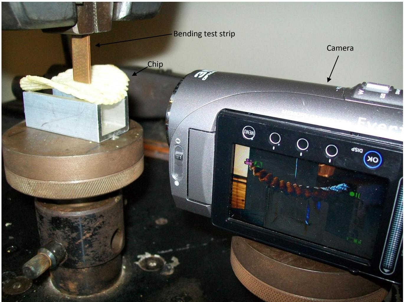
*Figure 2 Set up for three point stress test. a chip is placed across the gap of a piece of aluminum with the video camera pointed at the trial.*
