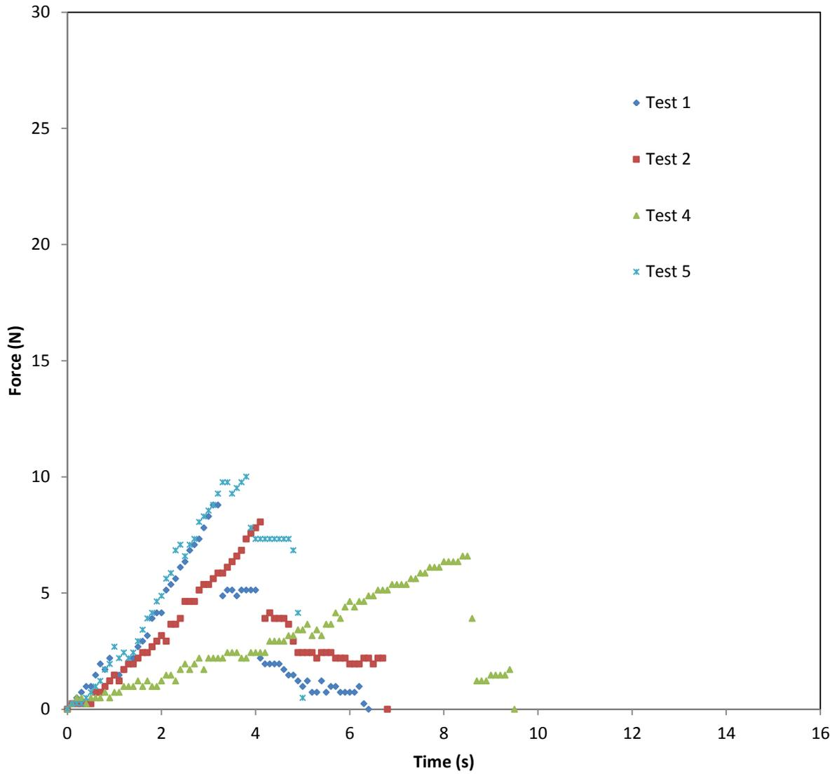
Figure 12 Force verse time graph for the four 3 point flexural test for Wise Ridgies chips. One trial was removed due to errors in data collection.
