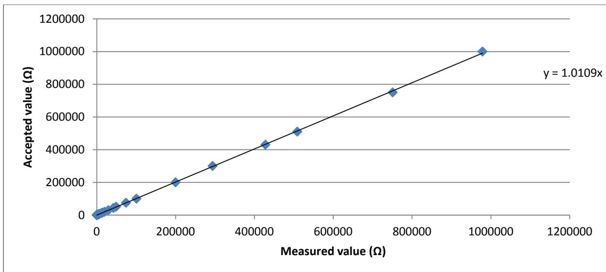
Figure 7 Calibration of the multimeter. Measured values were plotted with the accepted values of tested resistors. Following values given by the multimeter are inserted into the linear equation to account for error from the multimeter.
