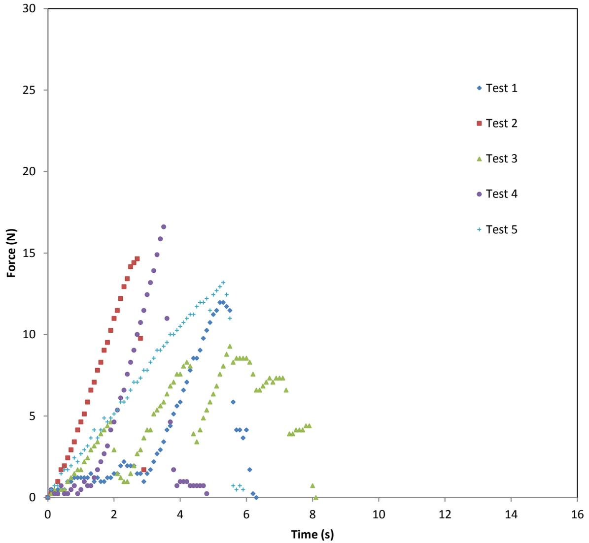
Figure 9 Force verse time graph for the five 3 point flexural test for Santitas Tortilla chips.
