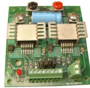
Figure 18: Simple-H Motor Controller
