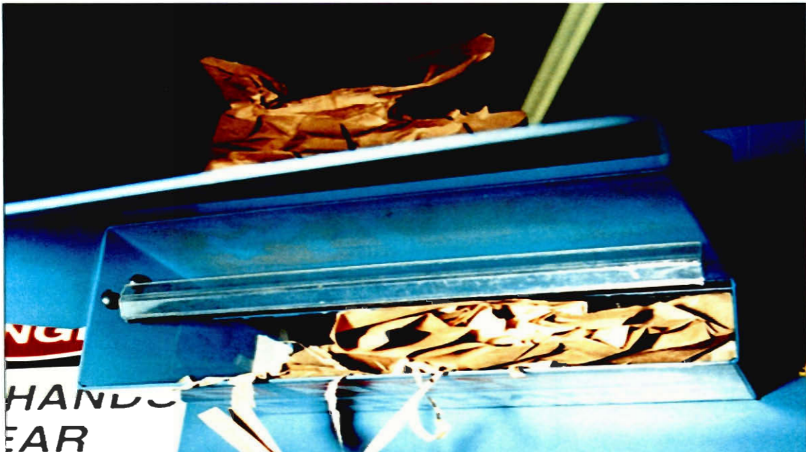
Figure 3.2: Photo of a Paper Jam in PADPAK Machine #1
