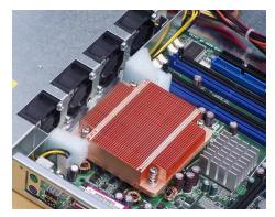
Figure 13: CPU air-cooler inside a server with fans [30].
