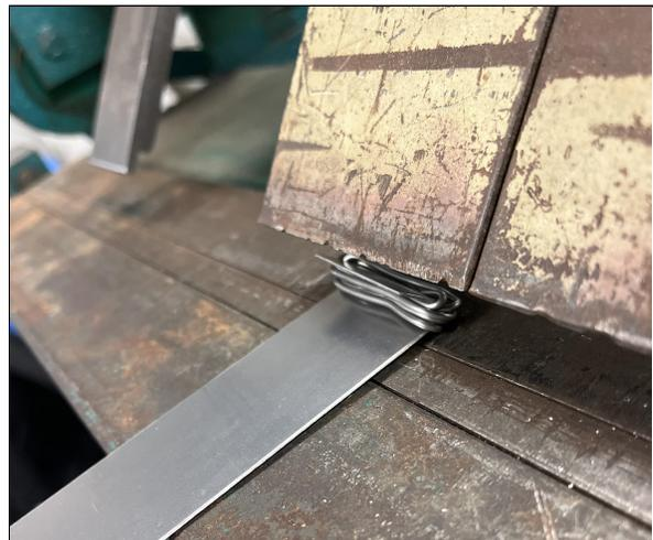
Figure 36: Sheet metal with spacer for second bend
