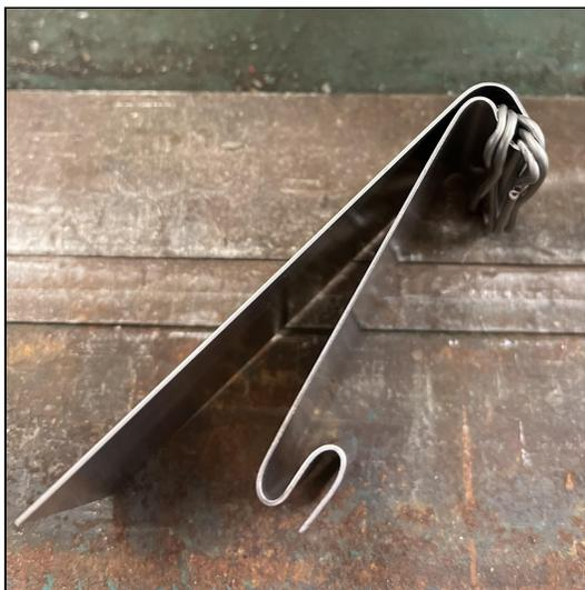
Figure 40: Flat spring with excess material and spacer
