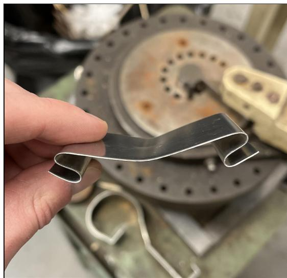
Figure 43: Flat spring with all bends as designed
