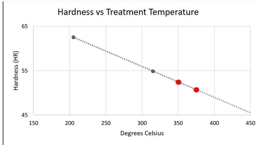
Figure 27: Hardness vs. Heat Treatment Temperature Graph
