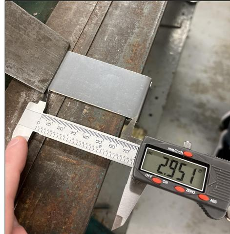
Figure 38: End of spring 2.95in from the brake bender
