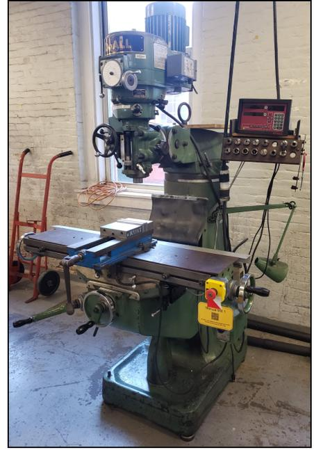
Figure 47: Manual Mill Machine
