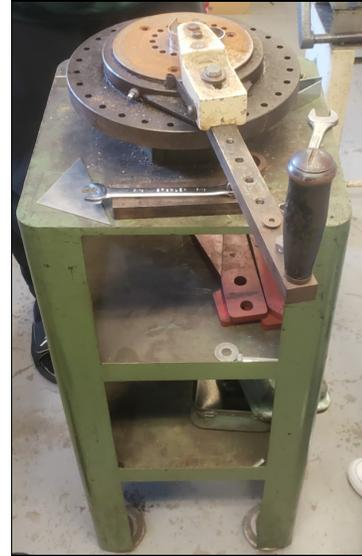
Figure 34: Image of Tube Bender
