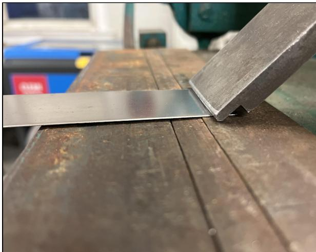
Figure 35: Sheet metal under brake bender
