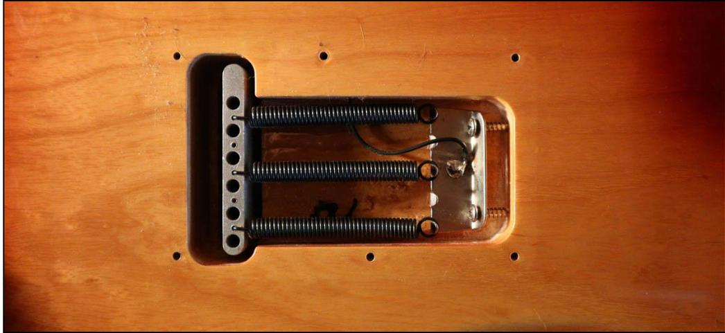
Figure 2: Typical spring system for a guitar's vibrato system
