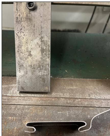
Figure 41: Flat spring with excess material unbent
