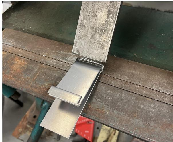
Figure 39: Second S bend with spacer
