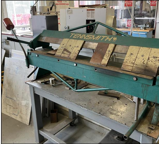
Figure 33: Image of Tennsmith Brake Bender
