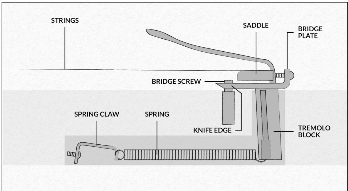
Figure 3: Diagram of the entire typical vibrato system
