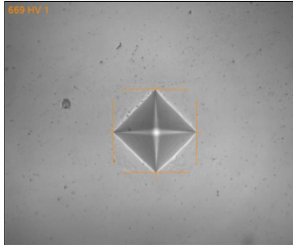
Figure 25: Hardness Testing using a Vickers indenter
