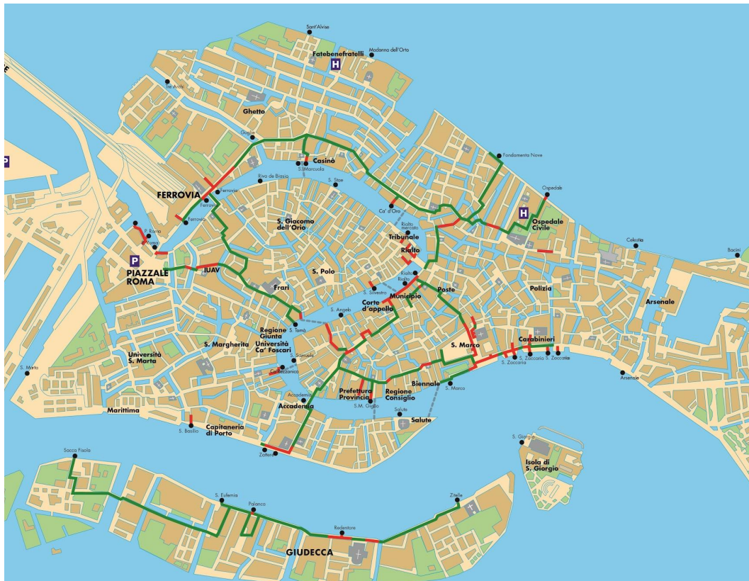
Figure 7: Raised walkways that remain dry at tides +120 cm (Municipality of Venice, 2016).
