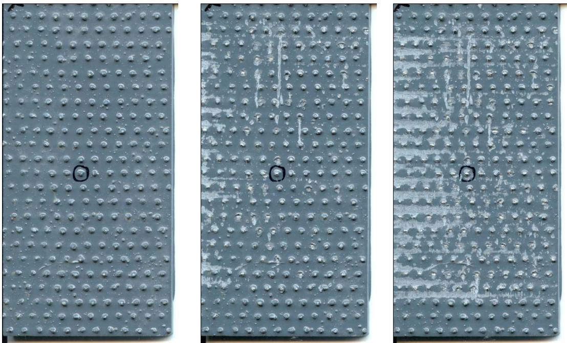
LDN 5086: Pre-Wear, 50 Cycles of Wear, 500 Cycles of Wear
