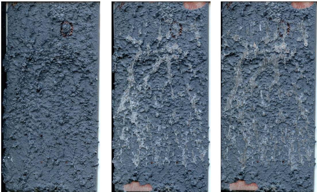
LDN A36: Pre-Wear, 50 Cycles of Wear, 500 Cycles of Wear
