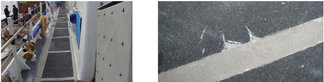
Figure 2: Peel and Stick Non-Skid, 110' Patrol Boat (left), Edge Failure (right)
