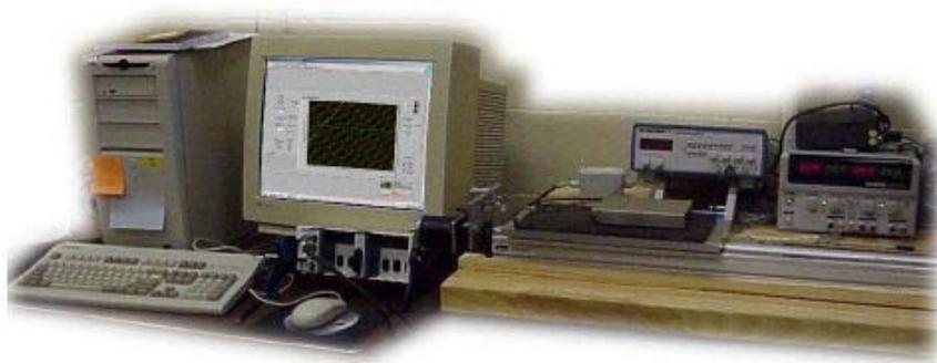
Figure 14: COF Measuring Apparatus
