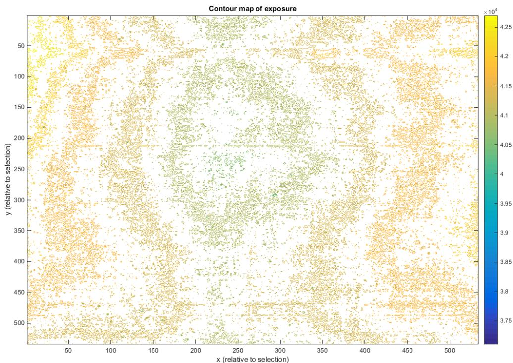
**Figure 3: Gafchromic film placed on beam spot**
