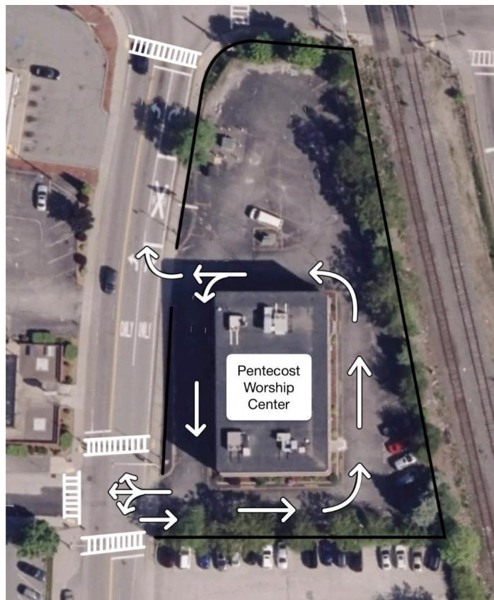
Figure 16: Traffic flow diagram at the Pentecost Worship Center parking lot.
