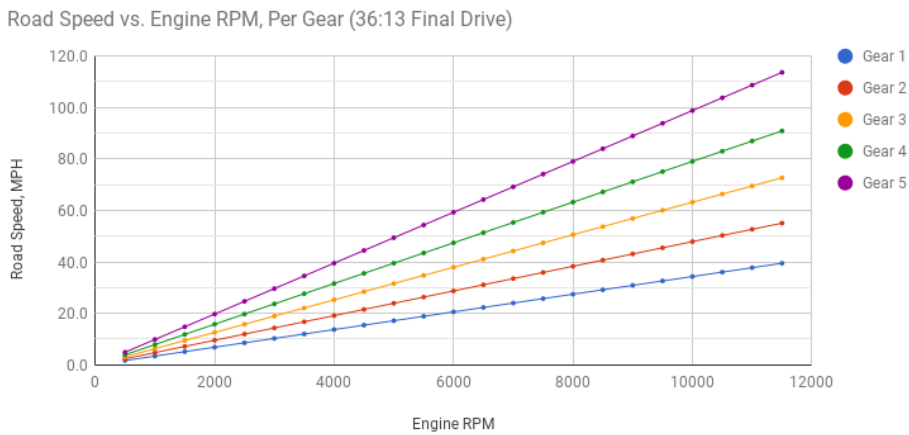
Figure 10: Chart of Road Speed vs. RPM for 36:13 Final Drive with WR450F
