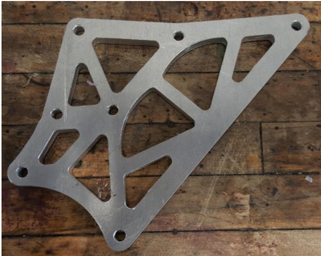
Figure 59: The new side panel design
