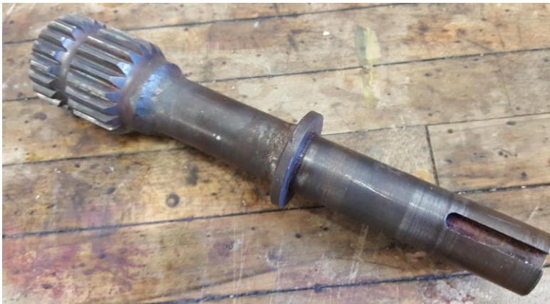
Figure 55: Steering shaft from the steering wheel to the steering box.
