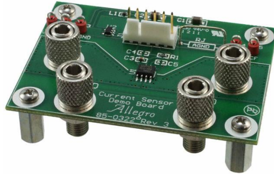
Figure 24: The current sensing hall-effect board.
