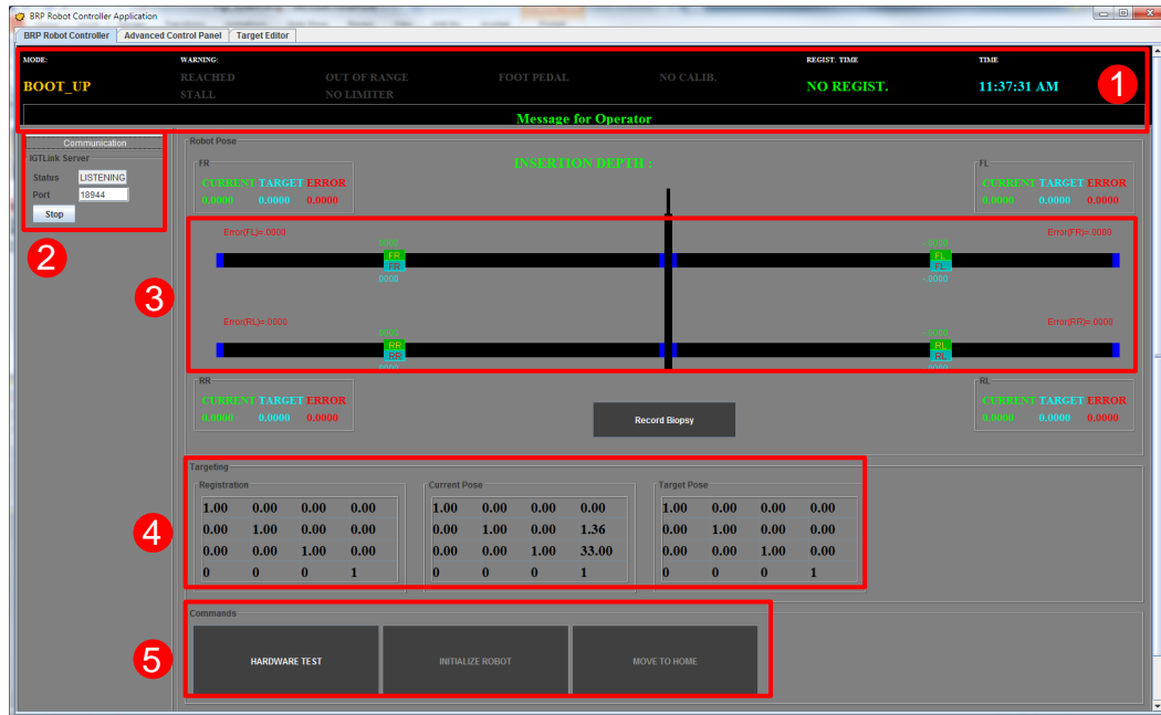
Figure 3.9: Clinical robot control application (CUI) showing: (1) robot status information, (2) OpenIGTLink connection status with the navigation application, (3) current and target robot joint positions, (4) robot pose, registration transform and target transform and (5) control buttons for robot hardware test and initialization.
