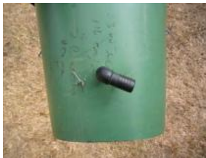
Figure 46. Fitting Pipe Bend to Bucket (Morgan, 2007)
