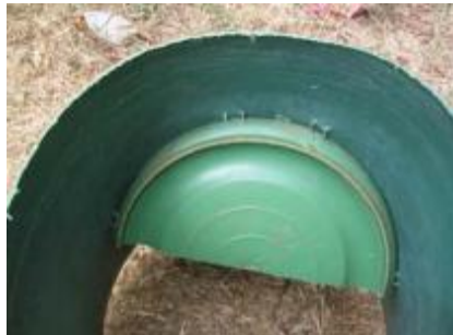
Figure 45. Attached Diverter with Wire (Morgan, 2007)
