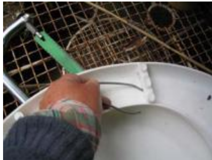
Figure 48. Using Hot Wire to Make a Hole through the Plastic Toilet Seat Ribs (Morgan, 2007)
