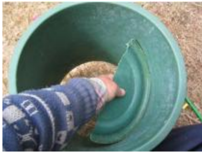
Figure 44. Placing Urine Diverter (Cut Base Half) Half-way up Bucket at an Angle (Morgan, 2007)
