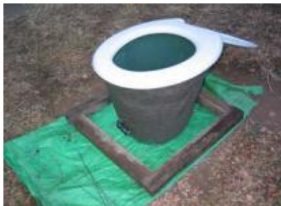
Figure 55. Bucket and Seat within Base Mould (Morgan, 2007)
