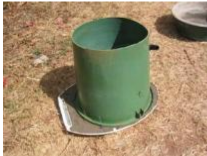
Figure 51. Bucket Fitted to Toilet Seat (Morgan, 2007)
