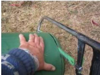
Figure 41. Cutting off the Bucket Base (Morgan, 2007)
