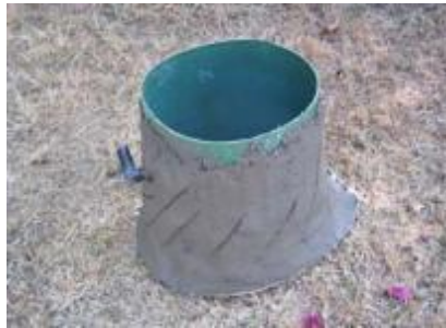
Figure 54. Concrete Added to the Second Half of Bucket (Morgan, 2007)
