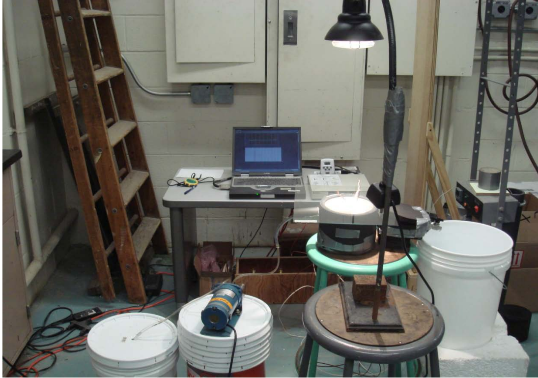
Figure C-7 Tinted glass placed on top of asphalt sample
