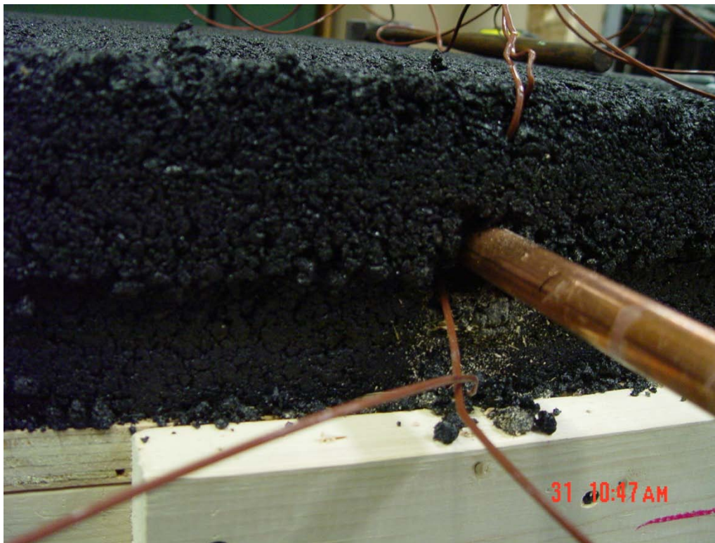
Figure G-6 Close-up of slab showing copper tube and thermocouples at different depths
