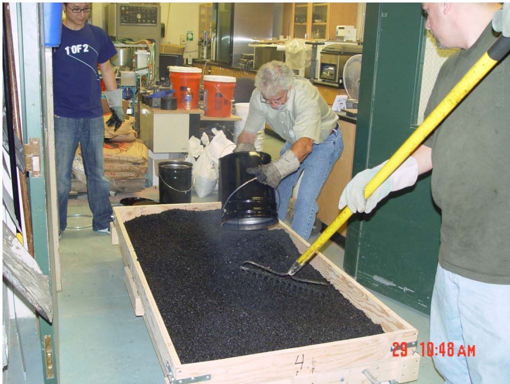
Figure G-2 Lay down of mix
