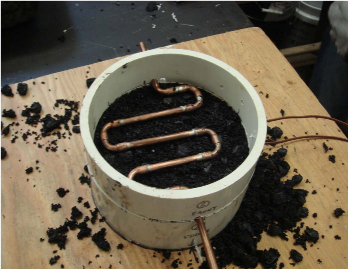
Figure 7-2 Serpentine pipe being placed and compacted
