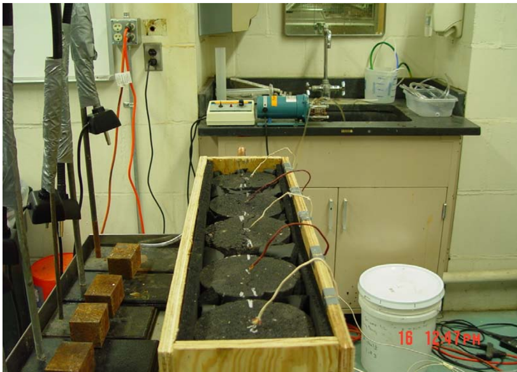
Figure C-4 Complied 5 asphalt pavements testing without halogen lamp on
