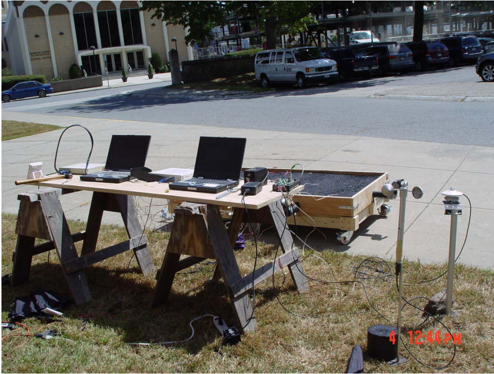
Figure G-7 Completed slab ready for testing
