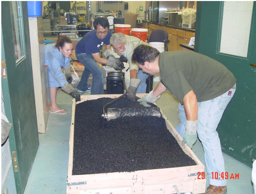
Figure G-3 Compaction
