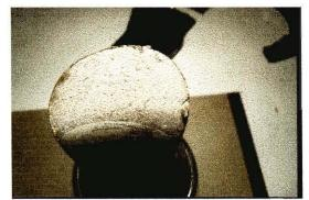
The above picture shows the small pimple that was put there by the setscrews. There is also another on the very bottom of the cross section of the shaft. This picture also shows that the lower section of the shaft is smoother than the top part of the shaft. This is a result of the fatigue failure. As the small crack grew it rubbed against the other part of the shaft and make it smooth. Then as the crack grew large enough the shaft fractured leaving the rest of the shaft rough.
