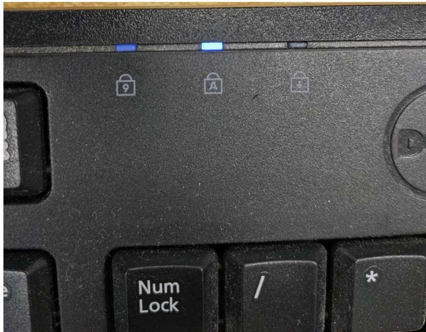
Figure 11: Keyboard from Lab Bench #23 has the scroll lock LED completely burnt out, and a dim num lock LED.
