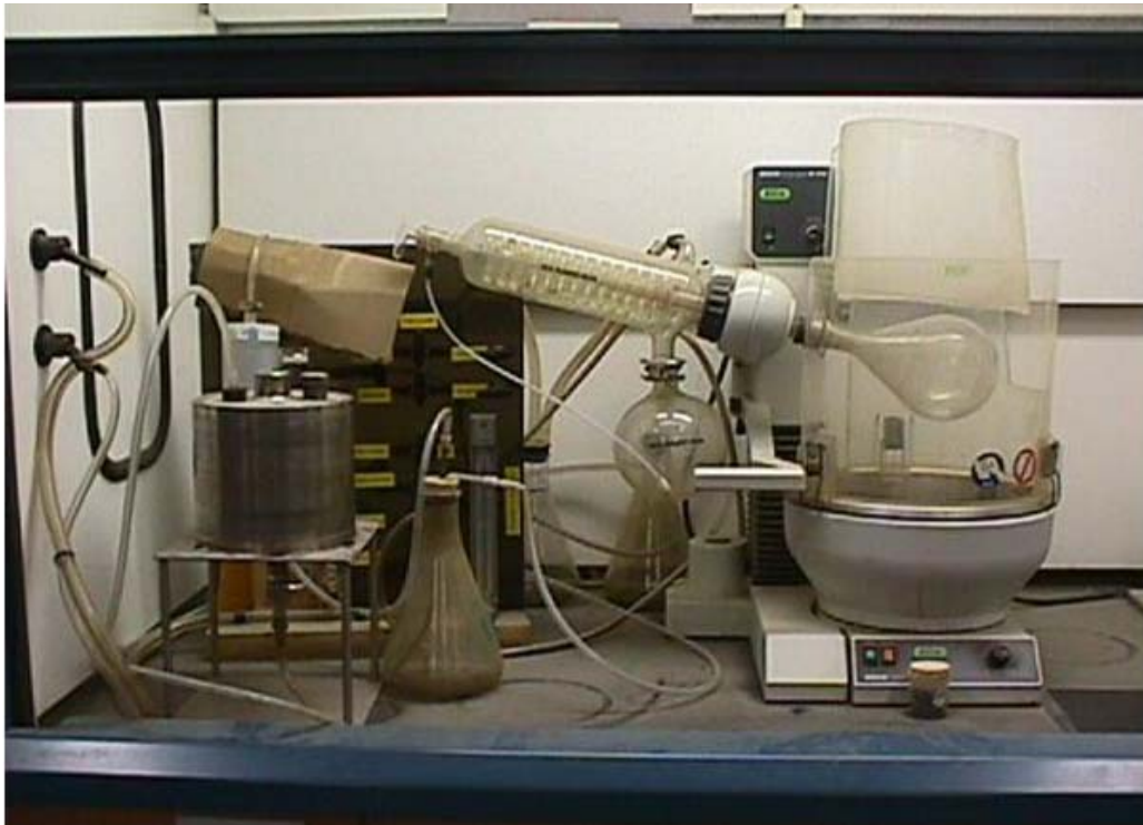
Figure 2.7. Asphalt Extraction Equipment Setup
