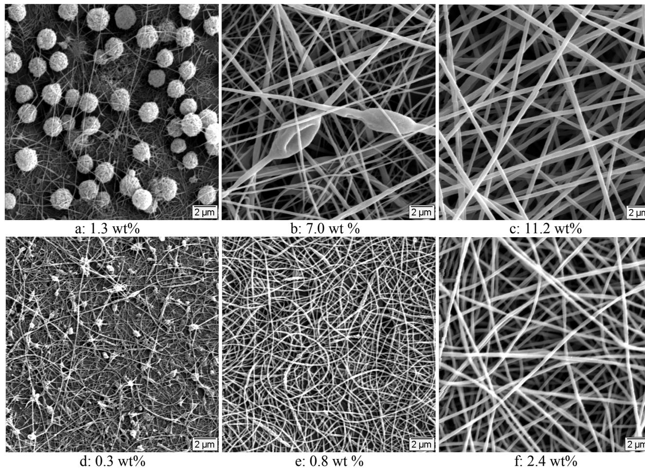
*Figure 10. Change in the morphology of high molecular weight polystyrene ((a, b, c): 1,045,000 g/mol, (d, e, f): 1,877,000 g/mol) electrospun from DMF. The corresponding solution concentrations are indicated.*
