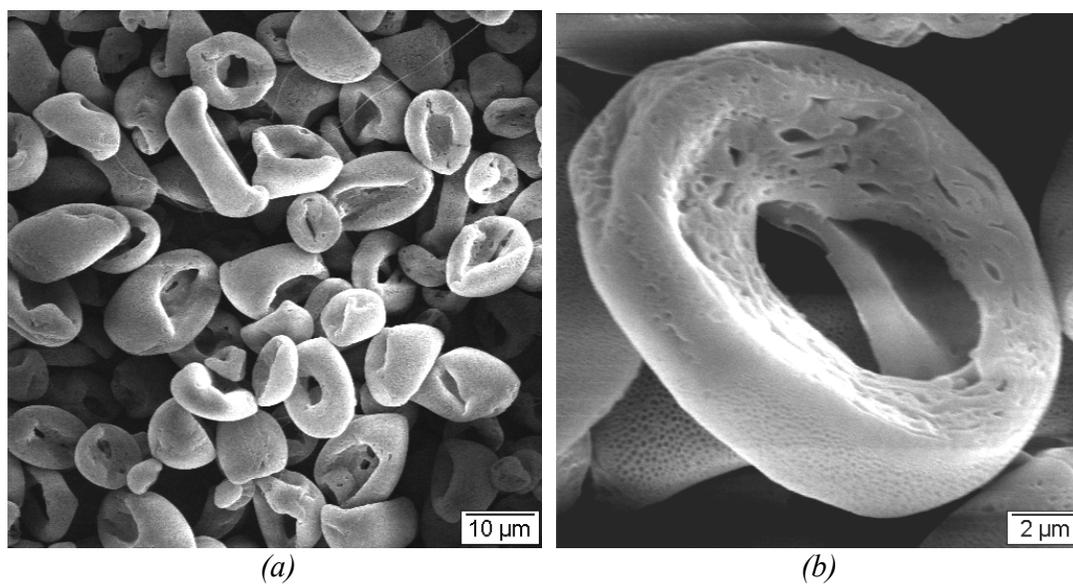
*Fig. 4. Photographs (a) showing the toroidal beads observed at  $M_w = 111,400$  g/mol and  $C = 6.3$  wt%. A high magnification photograph of a single toroidal bead is shown in (b).*
