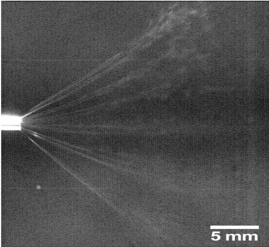
*Fig. 6. Photograph showing numerous minijets emerging from the capillary under steady-state conditions. The time elapsed after the initial jet emerged from the Taylor cone is 43.5 ms. (Solvent: THF,  $C = 0.072$  g/mL)*
