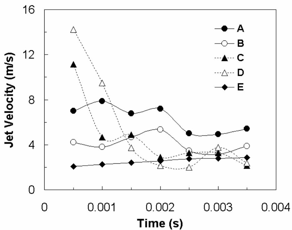
Fig. 16. Jet velocity as a function of time for various solvents. The time was measured after a stable jet emerged from Taylor cone. The typical standard deviation was around  $\pm 2$  m/s. (A: THF, B: chloroform, C: DMF, D: NMP, E: CS<sub>2</sub>)
