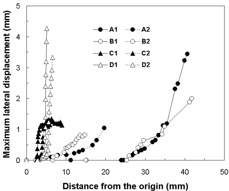
Fig. 18. Maximum size of the envelope cone formed during jet instability measured from a photograph. (A: THF, B: chloroform, C: DMF, D: NMP) Numbers 1 and 2 indicate primary and secondary jet respectively.
