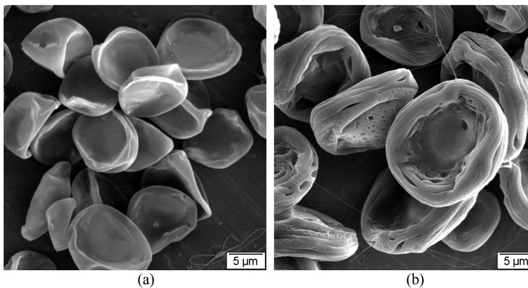
*Fig. 3. Photographs showing dish-shaped beads obtained with a)  $M_w = 19,300$  g/mol,  $C = 1.1$  wt% and b)  $M_w = 393,400$   $C = 3.3$  wt%. It can be noted that the dish-shaped beads in (b) have a greater wall thickness than in (a).*
