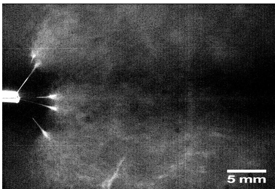
*Fig. 14. Photograph showing several jets emerging from the capillary under steady-state conditions during electrospinning with DMF as the solvent. The time elapsed after the initial jet emerged from the Taylor cone is 161 ms. ( $C = 0.071$  g/mL)*
