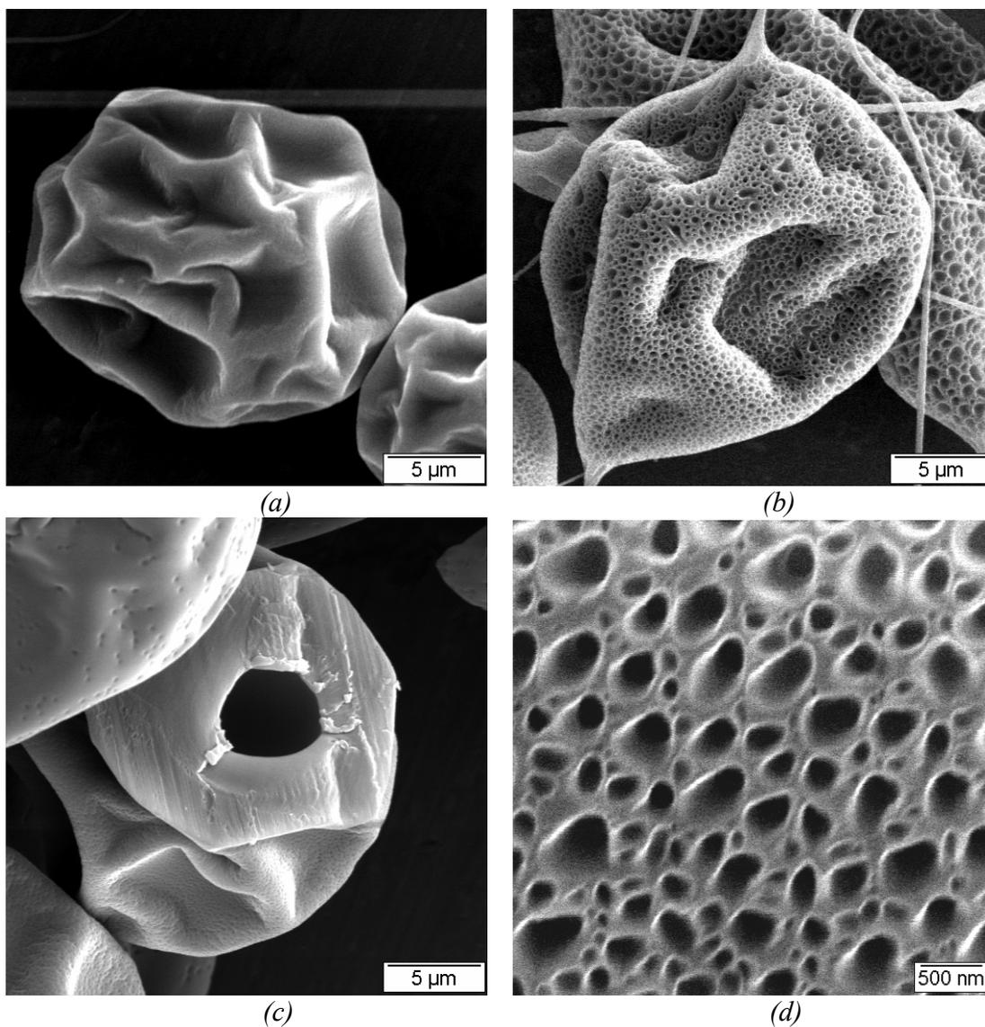
*Fig. 1* Photographs showing solid (a) and porous (b) wrinkled beads. The solid beads have been sliced to reveal a hollow structure inside (c). A high magnification photograph of the surface pore structure in porous beads (b) is shown in (d). ((a) and (c):  $M_w = 19,300$  g/mol,  $C = 32.4$  wt% (b) and (d):  $M_w = 393,400$  g/mol,  $C = 13.9$  wt%.)
