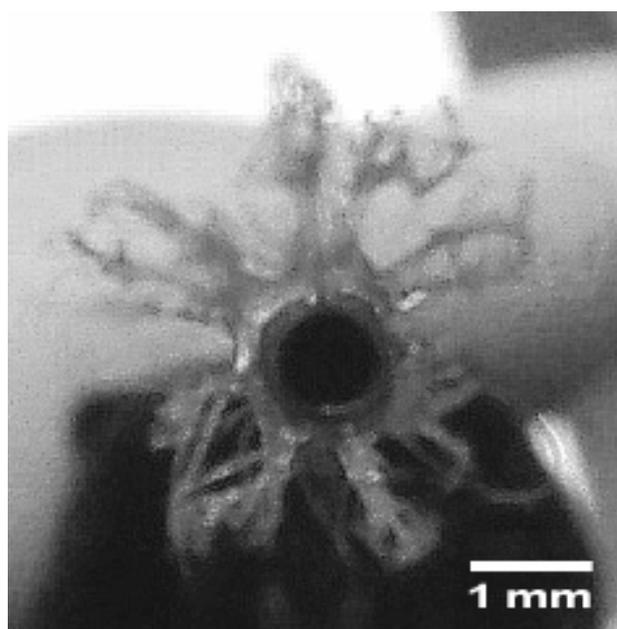
*Fig. 7. Photograph showing the tip of the needle at the end of the experiment. Numerous solidified fibers can be observed in the radial direction around the capillary edge. (Solvent: THF,  $C = 0.072$  g/mL)*
