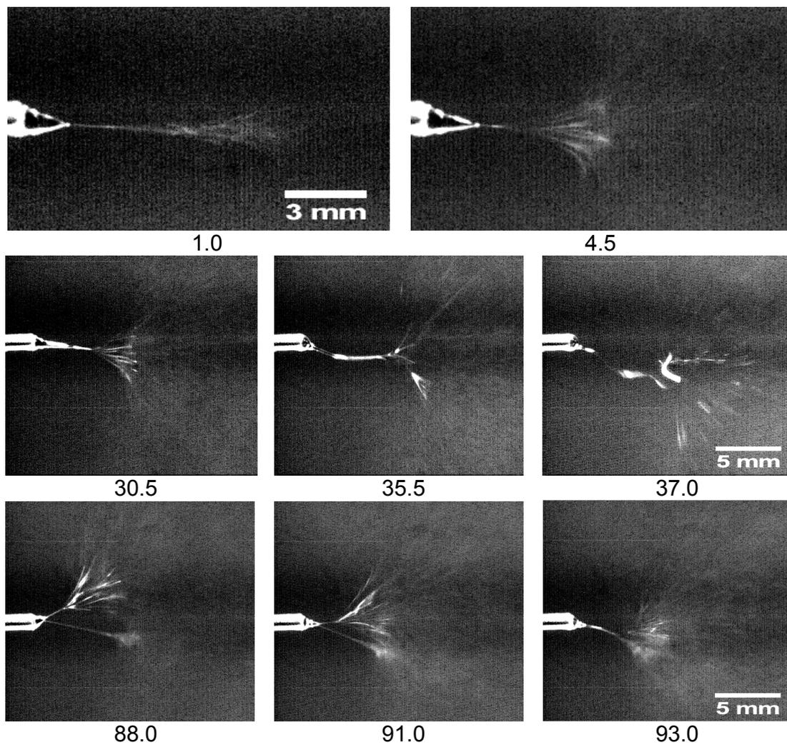
Fig. 13. Photographs showing the jet breakdown during electrospinning with NMP as the solvent. The numbers indicate the time elapsed (ms) after the jet emerges from the Taylor cone. ( $C = 0.071$  g/mL)
