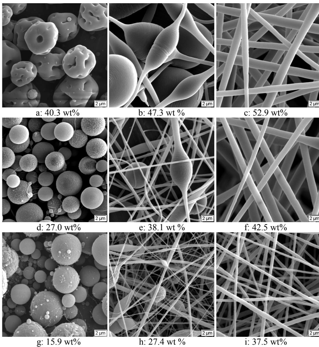
Figure 9. *Bead-to-fiber transition observed with low to moderate molecular weight polystyrene ((a, b, c): 19,300 g/mol, (d, e, f): 44,100 g/mol, (g, h, i): 111,400 g/mol) electrospun from DMF. The corresponding solution concentrations are indicated.*
