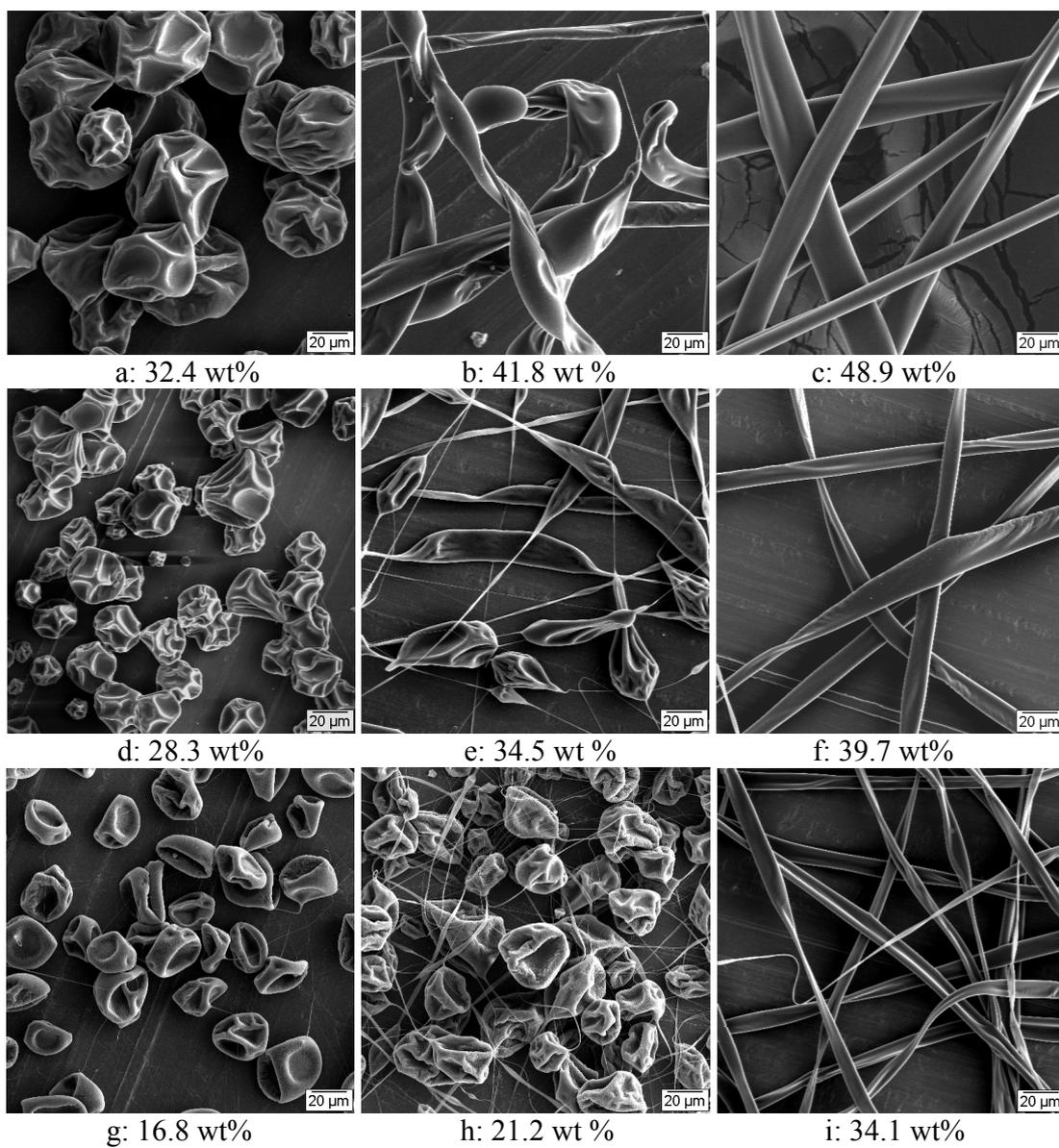
Figure 4. Bead to fiber transition observed with low to moderate molecular weight polystyrene ((a, b, c):  $M_w = 19,300$  g/mol, (d, e, f):  $M_w = 44,100$  g/mol, (g, h, i):  $M_w = 111,400$  g/mol) electrospun from THF. The corresponding solution concentrations are indicated.
