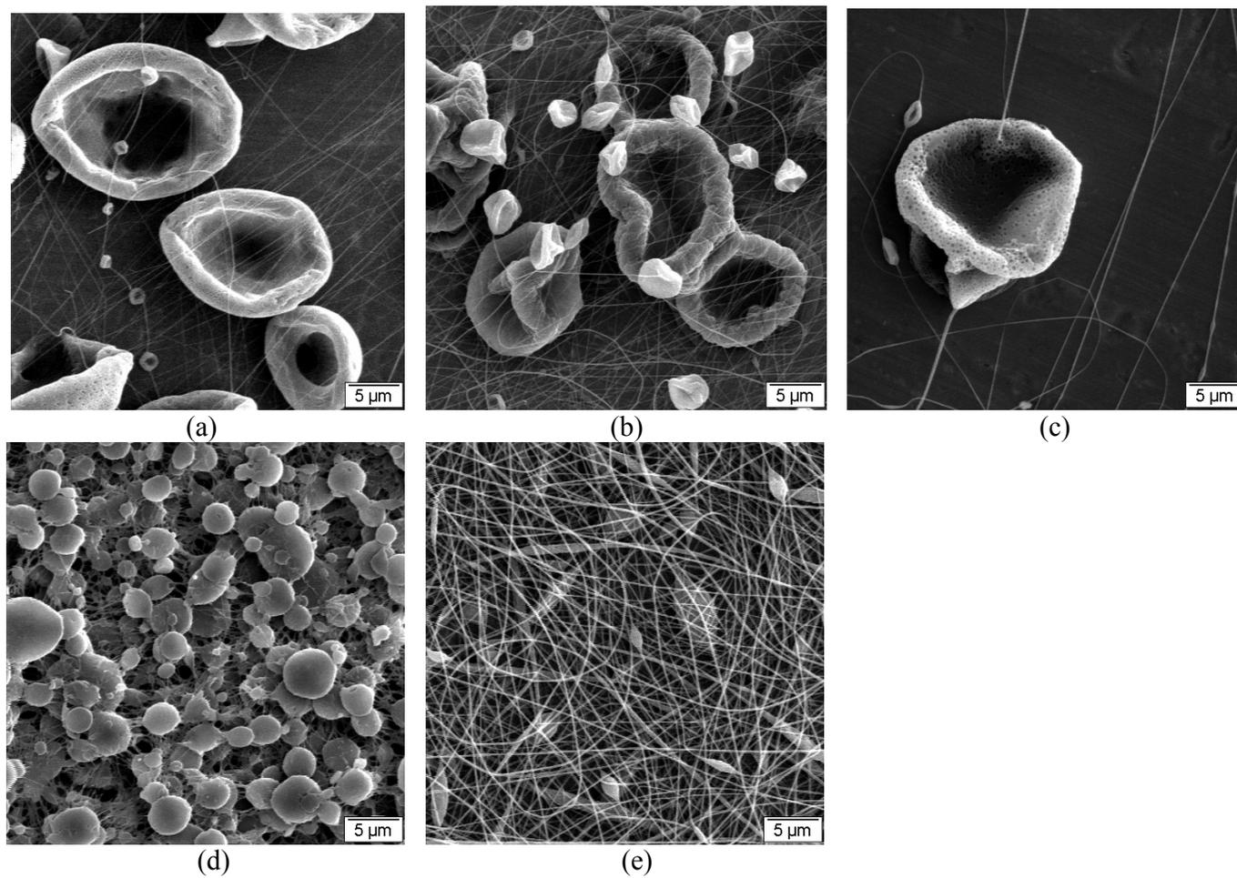
*Fig. 2. SEM photographs of polystyrene fibers and beads electrospun with various solvents (a: THF, b: Chloroform, c: CS<sub>2</sub>, d: NMP, e: DMF).*
