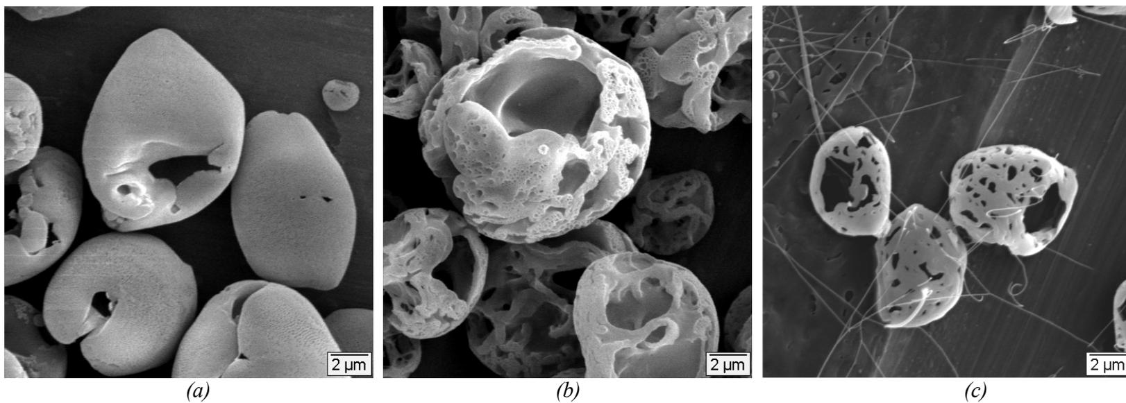
*Fig. 5. Photographs showing (a) hollow shells ( $M_w = 44,100$  g/mol,  $C = 2.6$  wt%), (b) micro-porous beads ( $M_w = 393,400$  g/mol,  $C = 2.6$  wt%) and (c) hollow porous beads ( $M_w = 1,877,000$  g/mol,  $C = 0.11$  wt%).*
