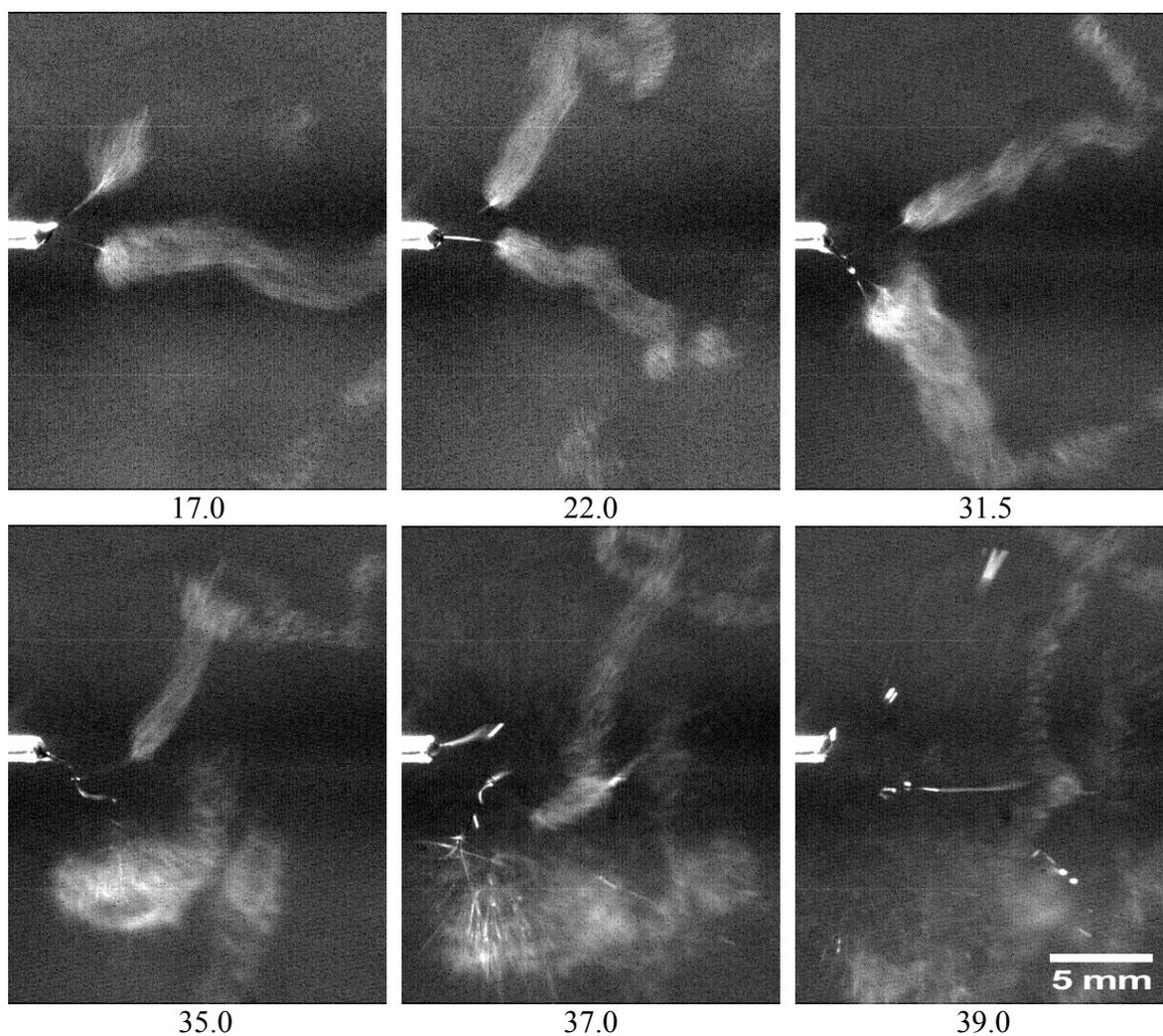
*Fig. 10. Photographs showing the development and breakdown of the secondary jet during electrospinning with DMF as the solvent. The numbers indicate the time elapsed (ms) after the jet emerges from the Taylor cone. Note the whipping instability that develops after 35.0 ms. ( $C = 0.120$  g/mL)*
