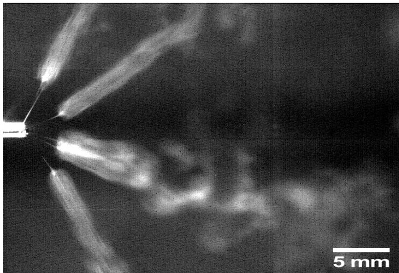
*Fig. 12. Photograph showing several jets emerging from the capillary under steady-state conditions during electrospinning with DMF as the solvent. The time elapsed after the initial jet emerged from the Taylor cone is 181.5 ms. ( $C = 0.120$  g/mL)*
