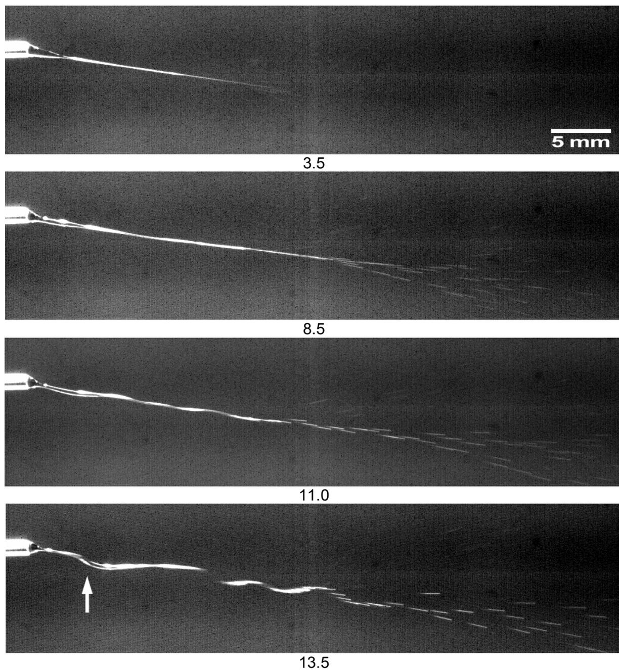
*Fig. 3. Sequential photographs showing the initial development of instabilities in the primary jet emerging from the capillary. The segment indicated by the arrow develops further jet instability shown in Fig. 4. The numbers indicate the time elapsed (ms) after the jet emerges from the Taylor cone. (Solvent: THF,  $C = 0.072$  g/mL)*
