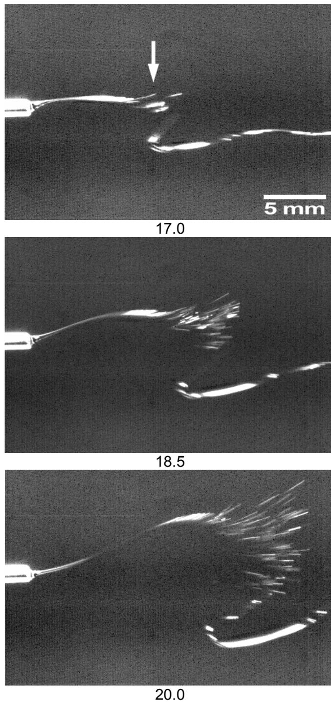
*Fig. 4. Images showing a growing perturbation leading to the breakup of the primary jet. The arrow indicates the loops created due to bending instability. The numbers indicate the time elapsed (ms) after the jet emerged from the Taylor cone. (Solvent: THF,  $C = 0.072$  g/mL)*
