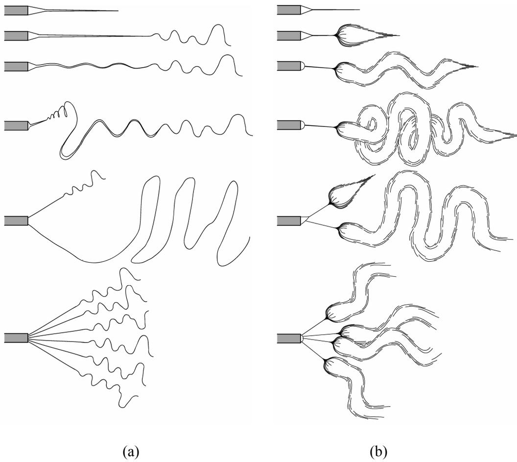
Fig. 17. Schematic of jet breakdown exhibited by two groups of solvent.
