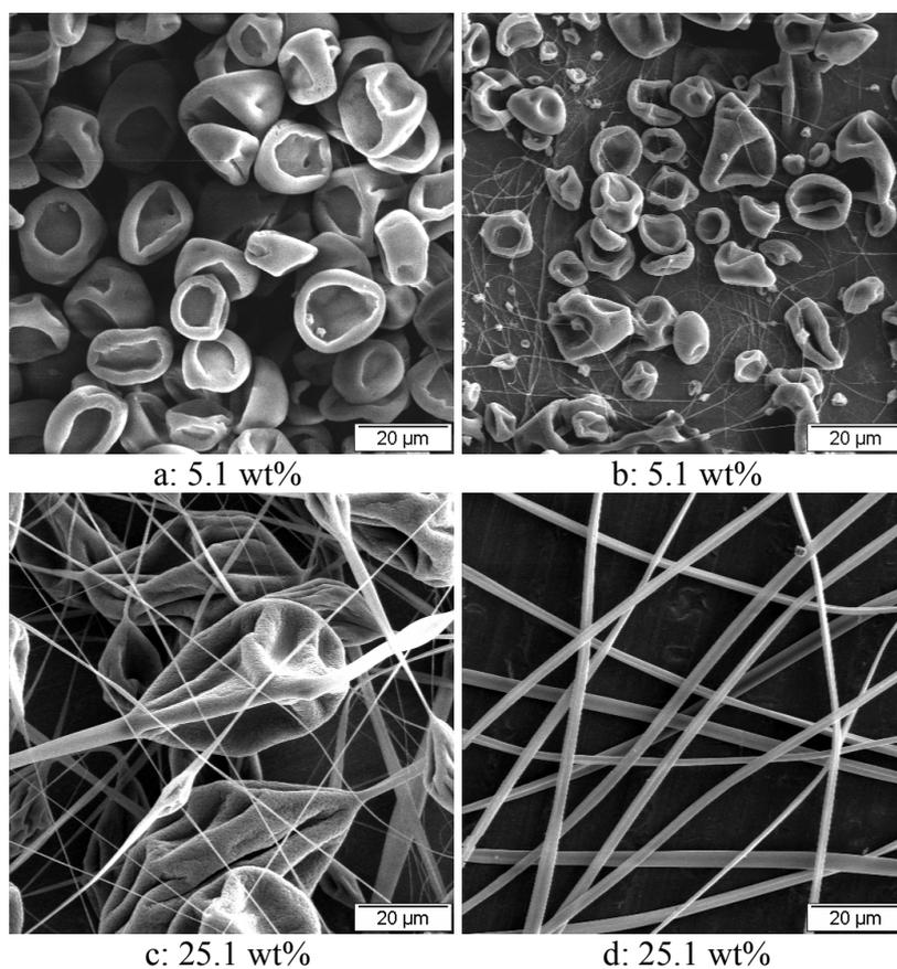
Fig. 3. SEM photographs showing the change in bead and fiber morphology with respect to applied voltage. Upon increasing the voltage from 10 kV (a, c) to 30 kV (b, d), fiber formation is facilitated. The corresponding solution concentrations are indicated ( $M_w = 111,400$  g/mol).
