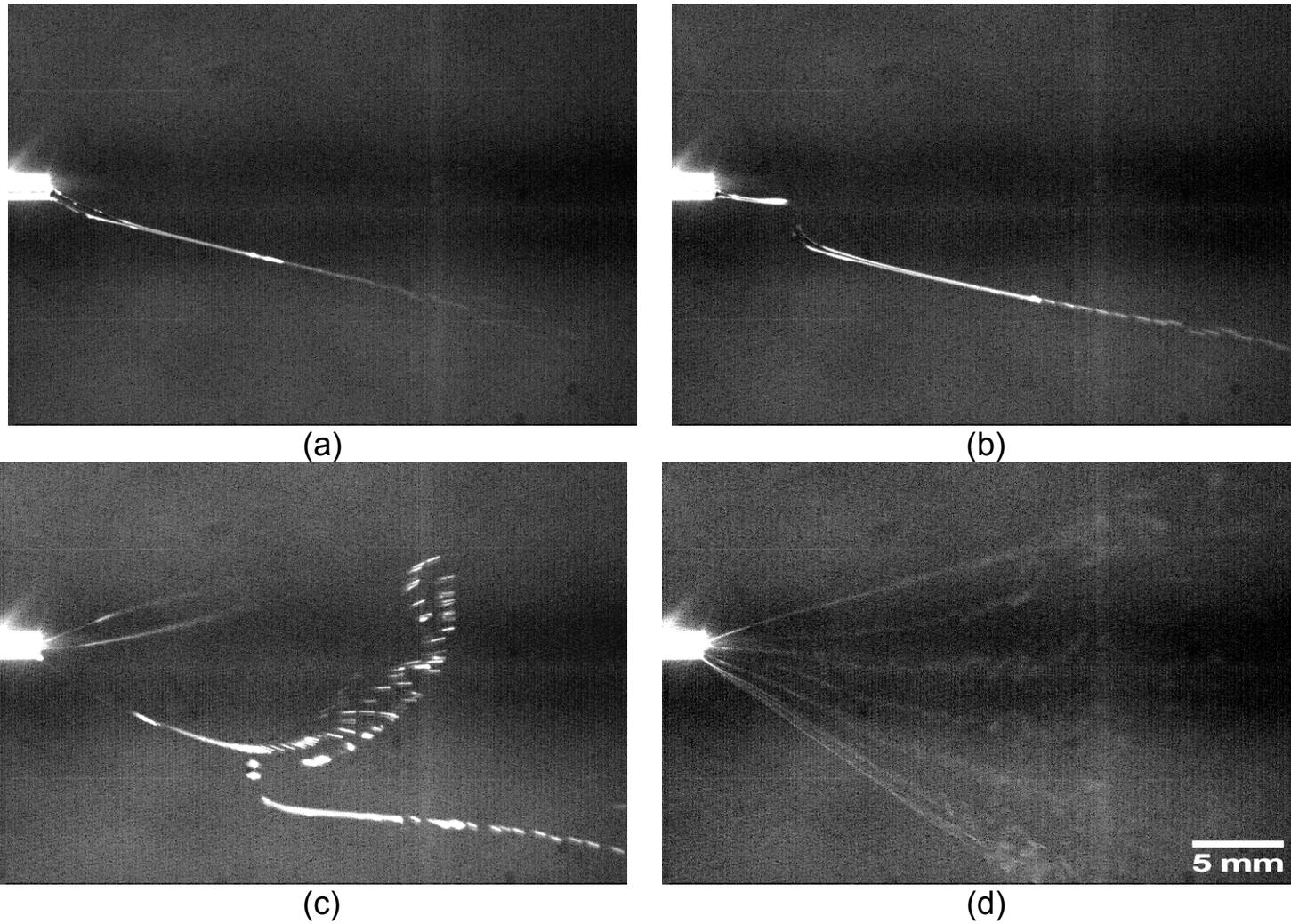
*Fig. 8. Photographs showing the jet development and breakup during electrospinning with chloroform as the solvent: (a) elongational flow, (b) development of bending instability, (c) breakup of primary jet and emergence of secondary jets, and (d) numerous jets under steady state. ( $C = 0.070$  g/mL)*
