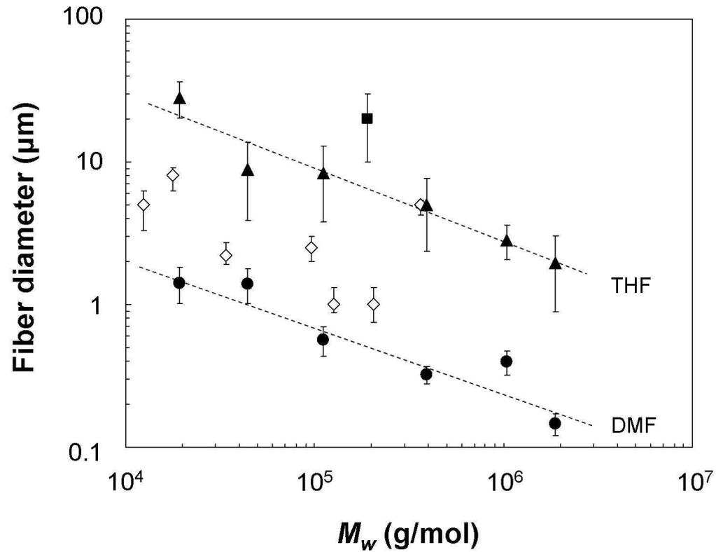
Figure 13. Average fiber diameter as a function of molecular weight for PS-THF and PS-DMF systems at the critical concentration,  $C_f$ , at which bead-free fibers are observed. The data of Megelski et al.[10] is indicated as a solid square (■). Relevant data of Gupta et al. [14], who examined PMMA-DMF system, are shown (as open diamond (◇)) for comparison.
