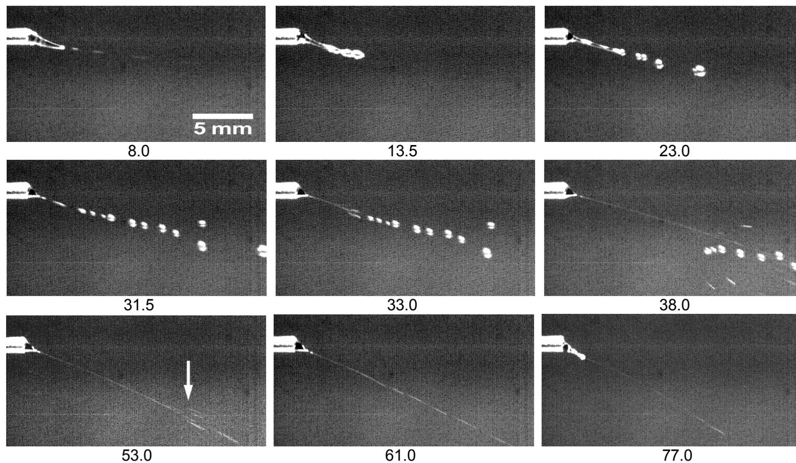
*Fig. 15. Photographs showing the jet breakdown during electrospinning with CS<sub>2</sub> as the solvent. The numbers indicate the time elapsed (ms) after the initial droplet emerges from the Taylor cone. The arrow indicates the breakup of a single steady state jet. (C = 0.072 g/mL)*
