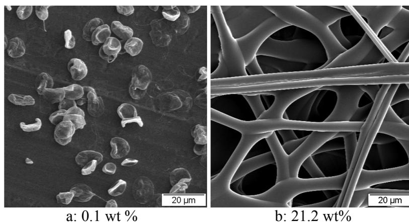
Fig. 2. Fused beads and fibers at (a) low and (b) high concentration ( $M_w = 393,400$  g/mol). The corresponding solution concentrations are indicated.
