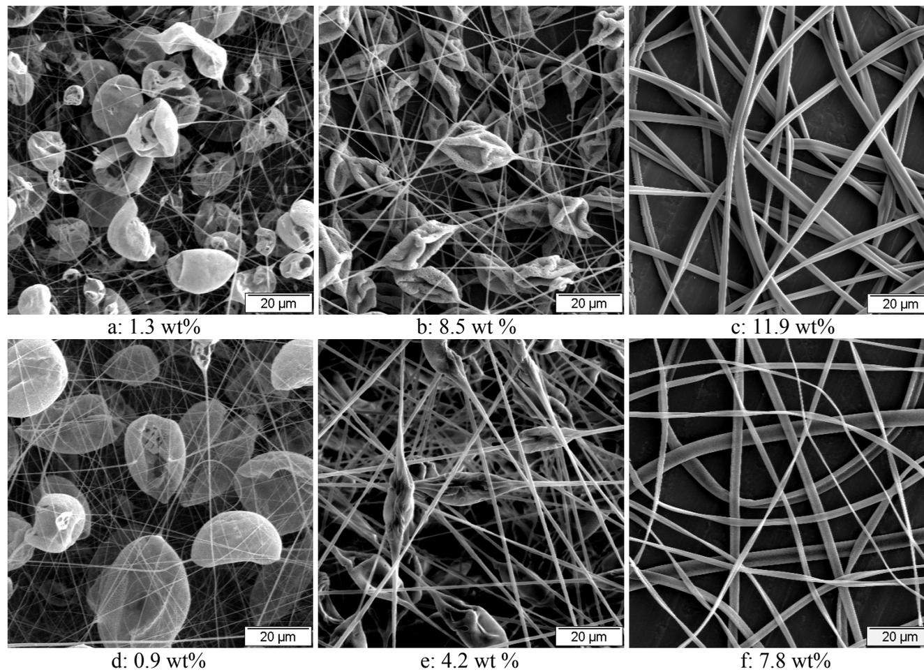
Figure 6. Change in the morphology of high molecular weight polystyrene ((a, b, c): 1,045,000 g/mol, (d, e, f): 1,877,000 g/mol) electrospun from THF. The corresponding solution concentrations are indicated.
