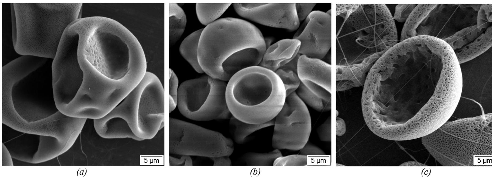
*Fig. 2. Photographs showing (a) dimpled beads, (b) non-porous cups and (c) porous cups. (a)  $M_w = 111,400$  g/mol and  $C = 13.9$  wt%, (b)  $M_w = 111,400$  g/mol,  $C = 11.8$  wt%, and (c)  $M_w = 393,400$  g/mol,  $C = 11.9$  wt%.*
