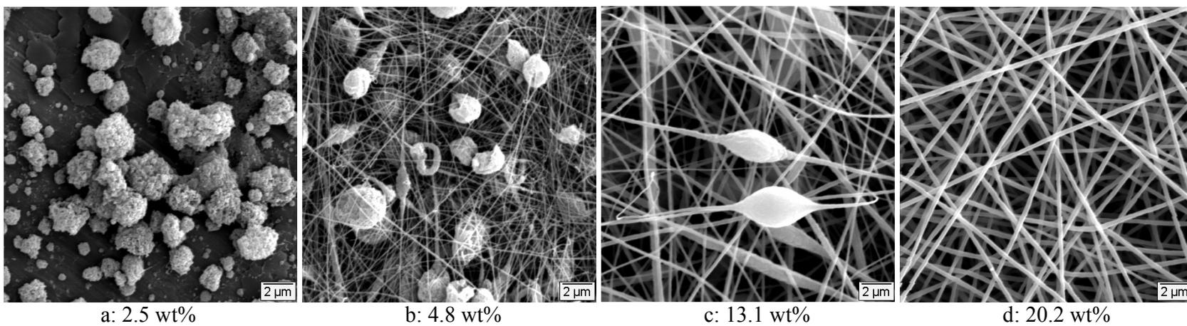
*Figure 8. Different structural regimes during bead-fiber transition of polystyrene electrospun from DMF. As the concentration is increased, the morphology consists of (a) beads only, (b) beads with incipient fibers, (c) bead-on-string, and (d) bead-free fibers. The corresponding solution concentrations are indicated.*
