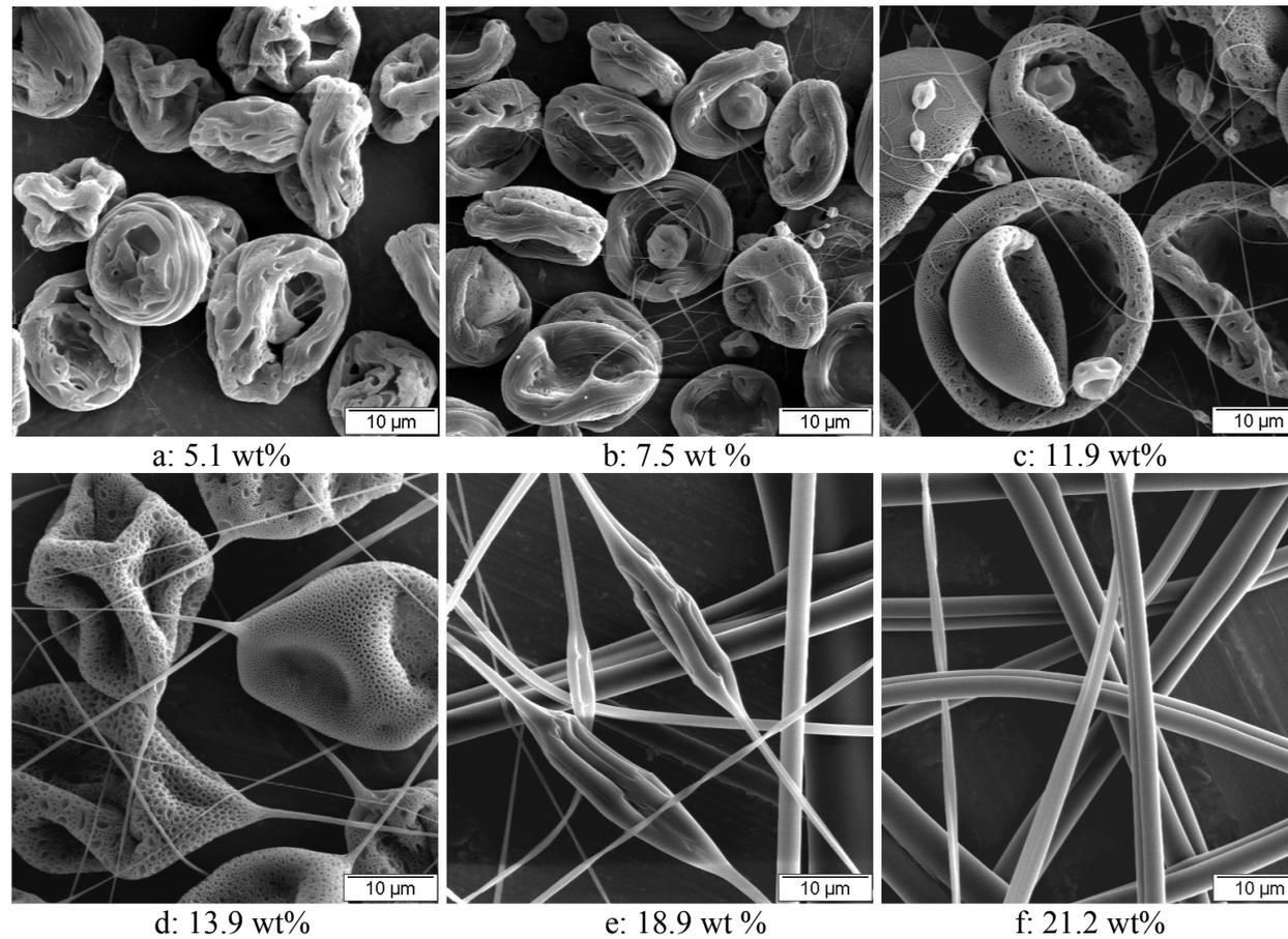
*Fig. 1. SEM photographs showing different structural regimes during bead-fiber transition. As the concentration is increased, the morphology consists of (a) beads only, (b,c) beads with incipient fibers, (d,e) bead-on-string, and (f) bead-free fibers ( $M_w = 393,400$  g/mol). The corresponding solution concentrations are indicated.*
