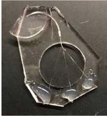
Figure 7-1. Construct for implantation sutures. Three threads are clamped into a bored out needle and were individually glued to the PDMS washer to facilitate seeding.
