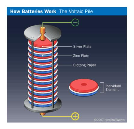
The Volata pile is what's known as a primary battery. That is to say it is constructed to produce a charge or a prescribed length of time. Once used up the cell must be rebuilt. In modern times think of the battery powering you remote control. The contrast to this will be discussed in the near future and is known as a secondary source. It has the ability and needs to be recharged periodically to keep producing a charge. In its most basic form, think of the starter battery in your car.
