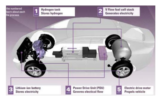
The storage tank contains hydrogen which is pumped through the fuel cell, sending energy to the lithium ion battery and drives an electric power train ( (FCX Claruty Power train, 2009). If the infrastructure could be efficiently implemented, we could see these cars on the road in the very near future. There are already a few on the road today in California. As this is new technology, it is also
