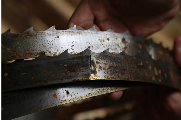
Figure 12: Band saw blade cracked from overuse
