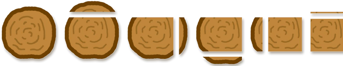
Figure 11: Five step milling process from log to squared off lumber
