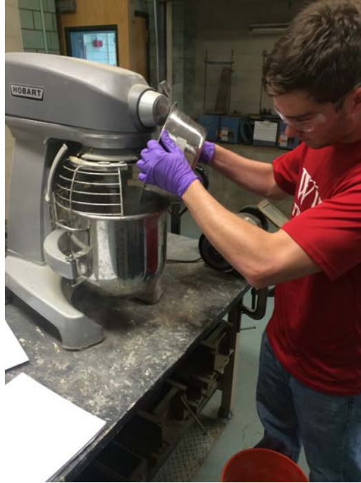
Figure 6 Materials being added to mixer
