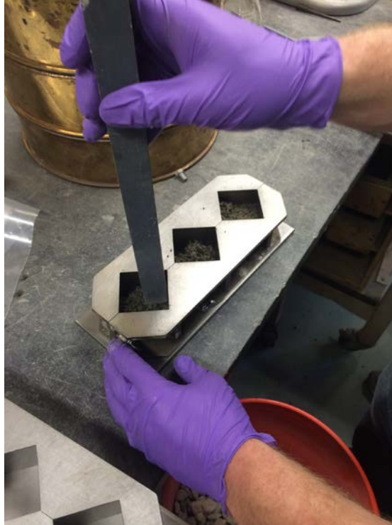
Figure 7 Rodding of cube samples
