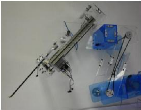
Fig. 4: First prototype of SASHA Research Platform, showing the da Vinci tool, links of the arm, and tool manipulation motors
