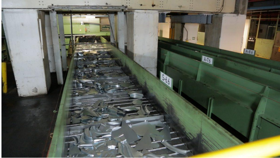
Fig. 2: Conveyor Transporting Aluminum Stamping Scrap.
