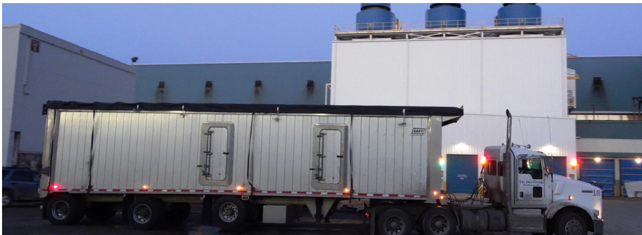
Fig. 6: Universal Trailers. Utilized by Ford to both deliver aluminum coil and take scrap. The trailers are loaded by the cyclone systems procedures that reduce expose to the environment [15].
