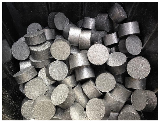
Fig. 21: Briquettes of Aluminum Dust.
