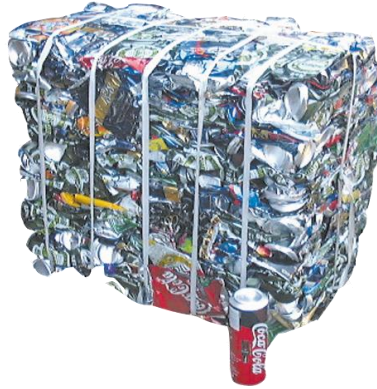
Fig. 20: Bale Composed of Crushed Aluminum Cans.
