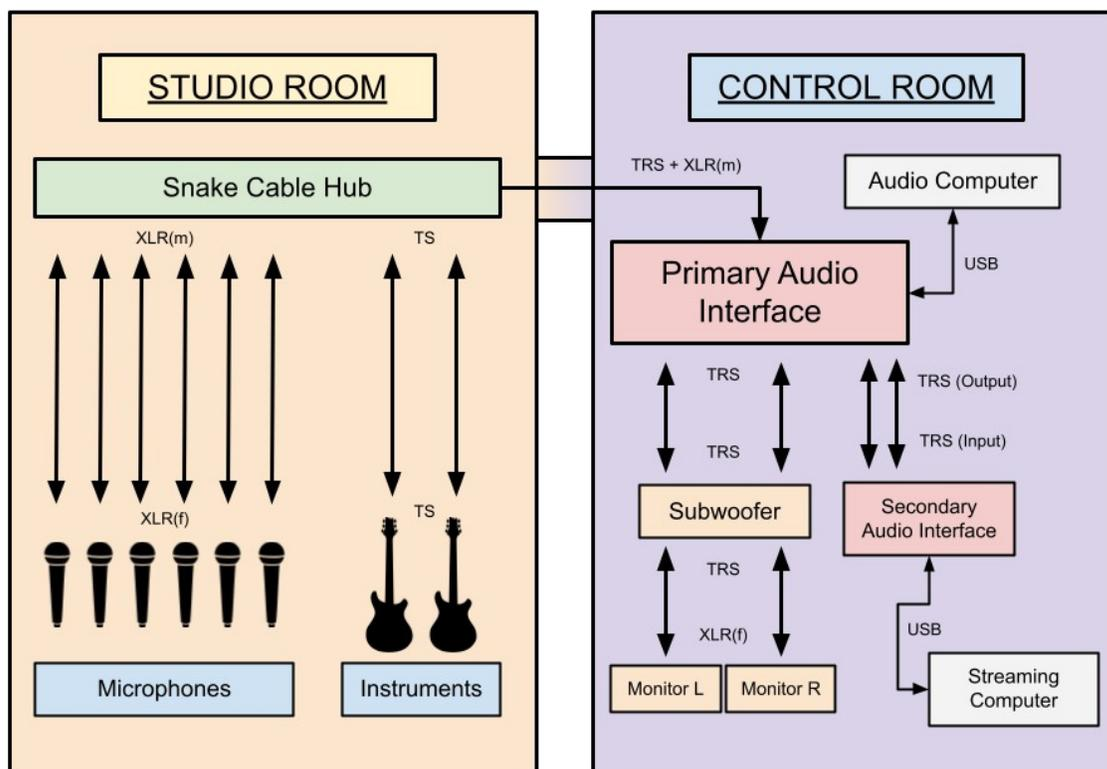
Figure 3.1: Audio Equipment Wiring Guide.
