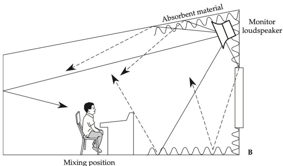
Figure 2.1: LEDE Control Room Conceptual Diagram. The side of the room with the loudspeaker is covered in absorptive material (the “dead” end), while the other is left reflective (the “live” end). Image Source: Everest and Pohlmann (2021).
