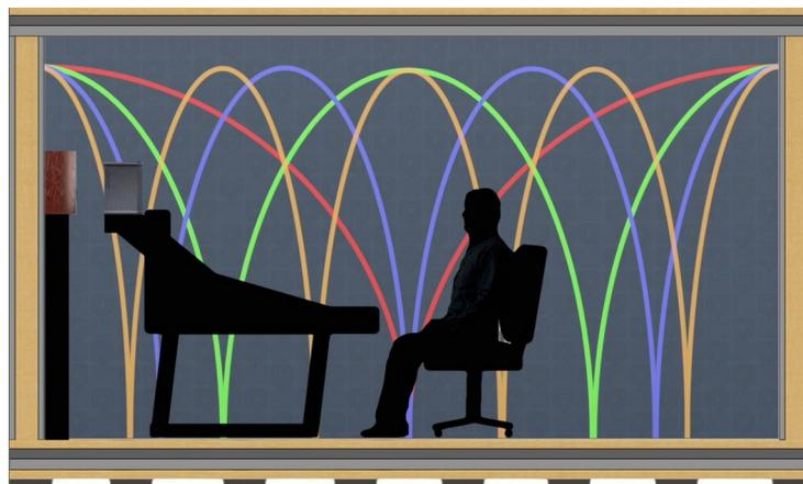
Figure 1.2: Standing Waves in a Studio Setting. The lines represent the intensities of the standing wave frequencies at each location. Image Source: Albano (n.d.)
