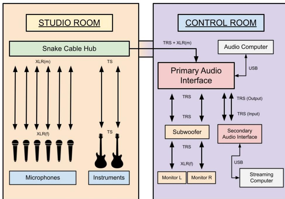
Figure B: Audio Equipment Wiring Guide
