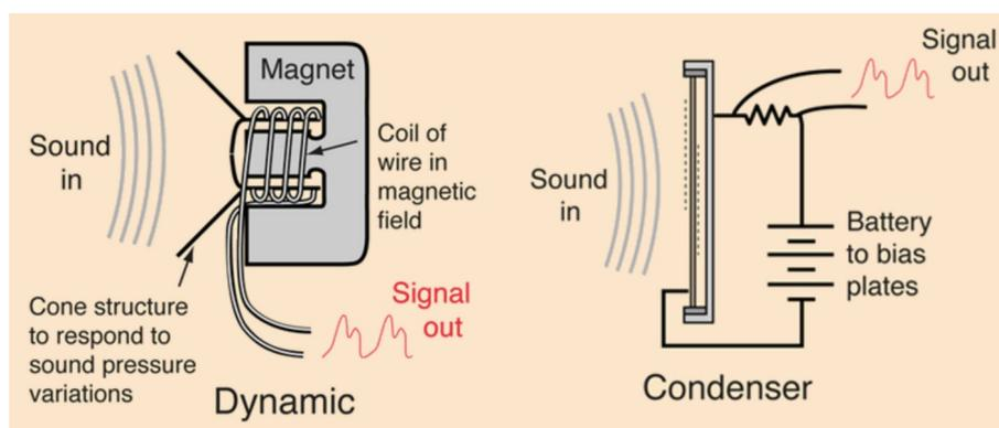
Figure 1.5: Diagrams of Dynamic and Condenser Microphones. Image Source: Nave (n.d.).
