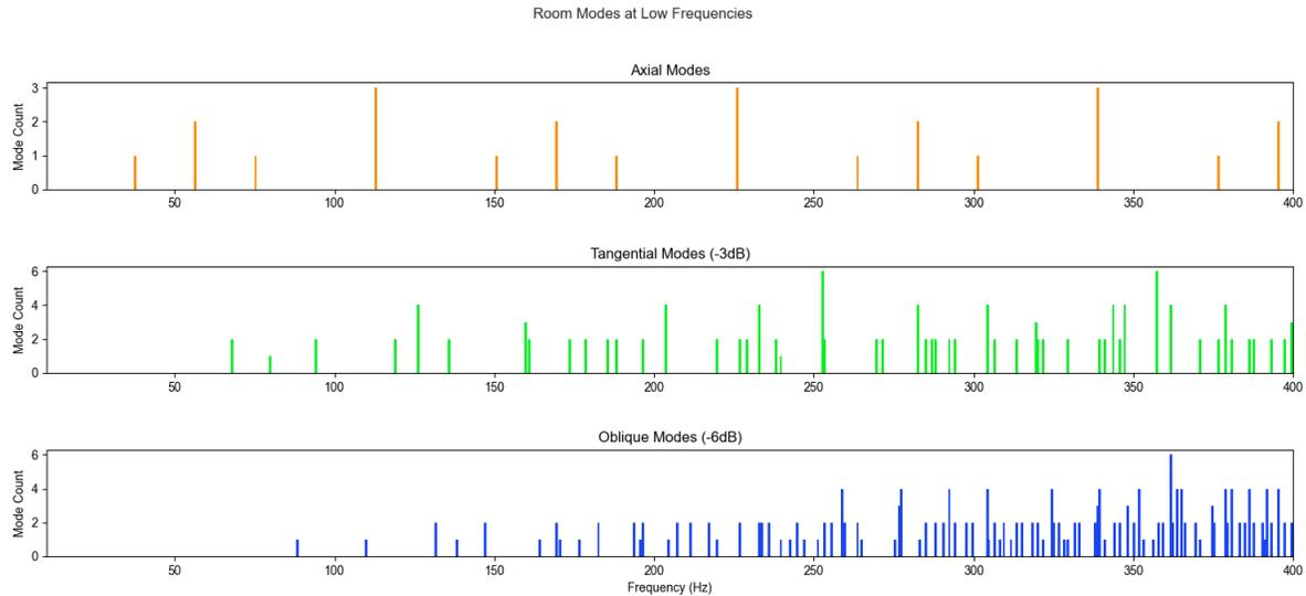
Figure 2.2: Room Modes Plot. Axial, tangential, and oblique room mode frequencies for a 10x15x10 ft room.
