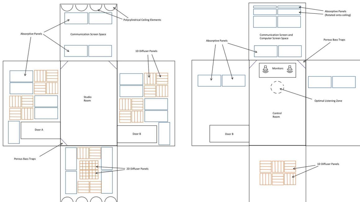
Figure 2.3: Acoustic Designs for the Studio and Control Rooms.
