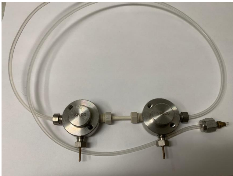
Figure 3-15: Sixth generation microreactor with a ceramic tube connector for increased mechanical integrity
