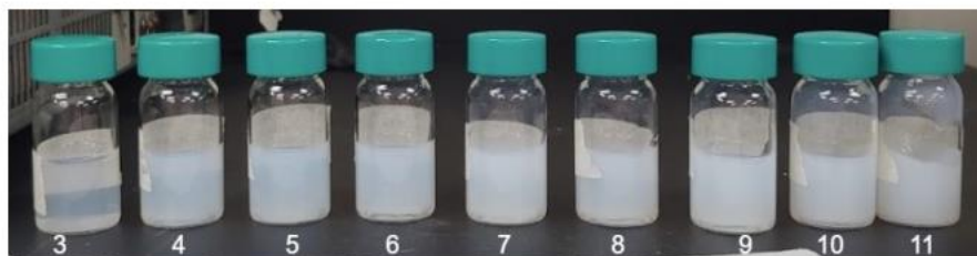
Figure 4-2: Visualization of the degree of polymerization of the support boehmite slurry as a function of the amount of hydrochloric acid added
