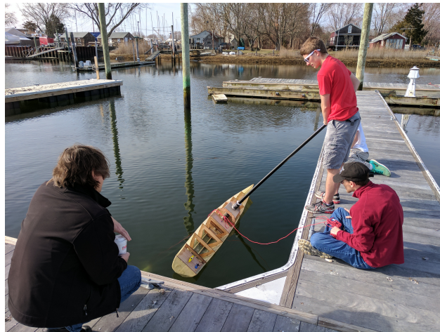
Figure 4.24: Keel Structure Testing Showing the Boat Heeled
