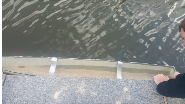
Figure 4.23: Hull Leak Test Showing a Small Leak
