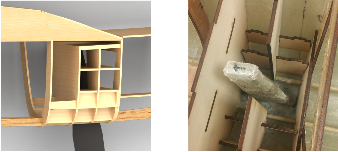
Figure 4.10: Keel Structure CAD vs. Actual Comparison View
