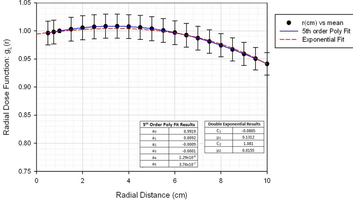
Figure 3: Calculated M-15 radial dose function,  $g_L(r)$ , at distance between 0.5 and 10cm with the resulting data fit to a fifth order polynomial and double exponential function
