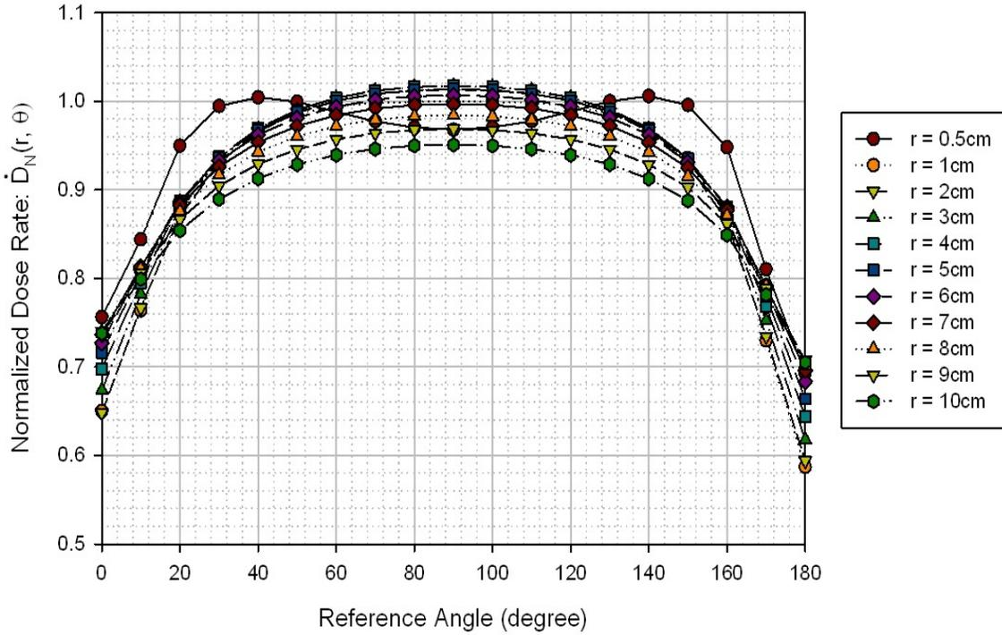
Figure 2: Presentation of the normalized dose rate distribution of model M-15 Iridium-192 from the MCNP output. Geometry effects were removed by multiplying the dose rate,  $\dot{D}(r, \theta)$ , by the radial distance squared,  $r^{-2}$ . Once corrected, the dose rate is then normalized to the dose rate at 1 cm along the seed's traverse's axis,  $\dot{D}(r_0, \theta_0) = 4.038 \pm 0.064 \text{ cGy mCi}^{-1} \text{ h}^{-1}$ , to obtain the normalized dose rate.
