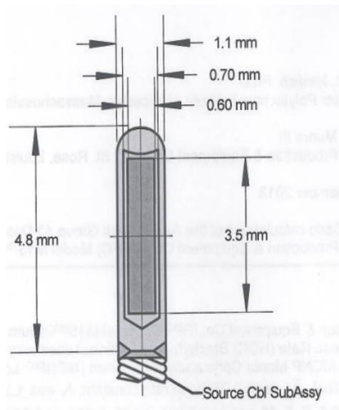
Figure 1: Configuration of the M-15 Iridium-192 HDR Brachytherapy source modeled for the MCNP simulation. This model consists of a 0.350cm long Iridium-192 source encapsulated in a steel shell
