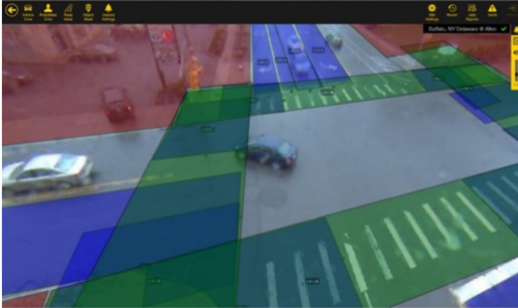
Figure 3: Perspective from camera showing detection zones (Baas, Galton, & Biton, 2016).
