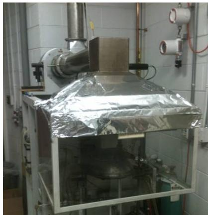
**Figure 6: Cone Calorimeter Adjustments for 175mm by 175mm Specimen**
