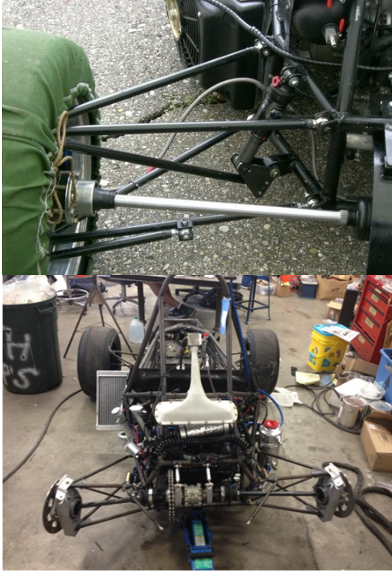
Figure 35 Example of Right Angle Control Arms
