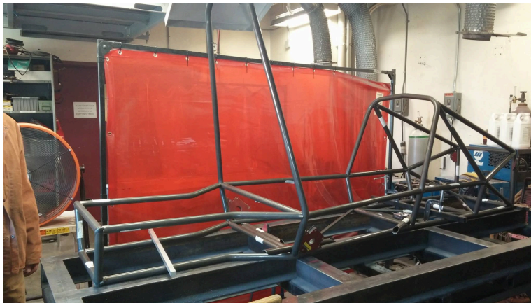
Figure 82 Main Roll Hoop Installed Free Standing
