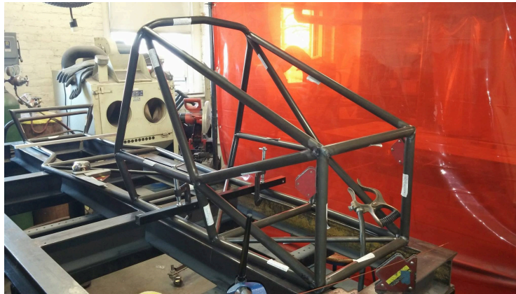
Figure 81 Fixturing of Front Drivers Cell
