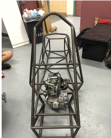
Figure 84 Frame Completed with Engine
