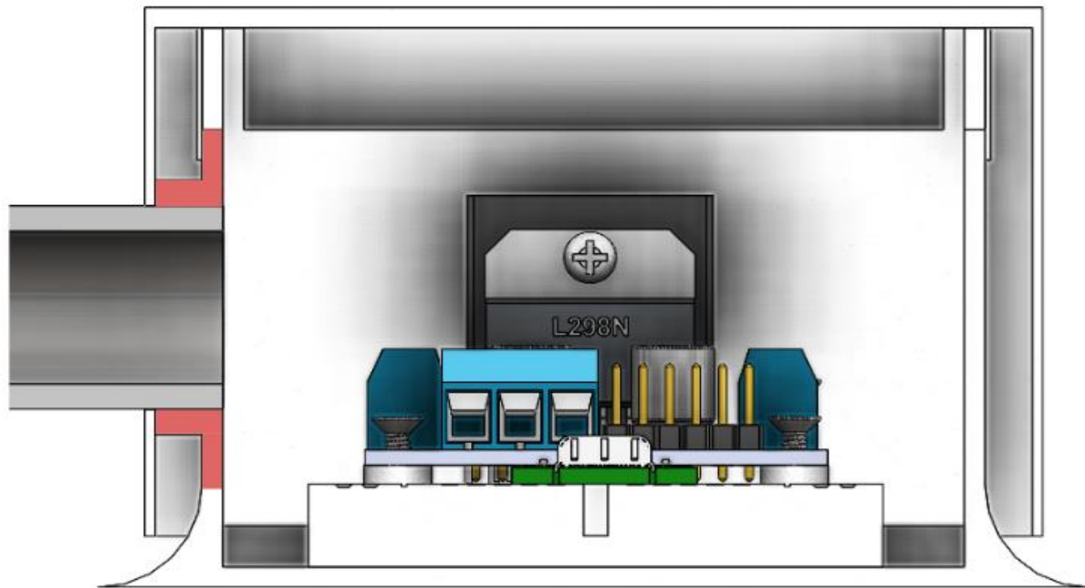
Figure 18: Extruded Wire Cover (highlighted in red) side view.
