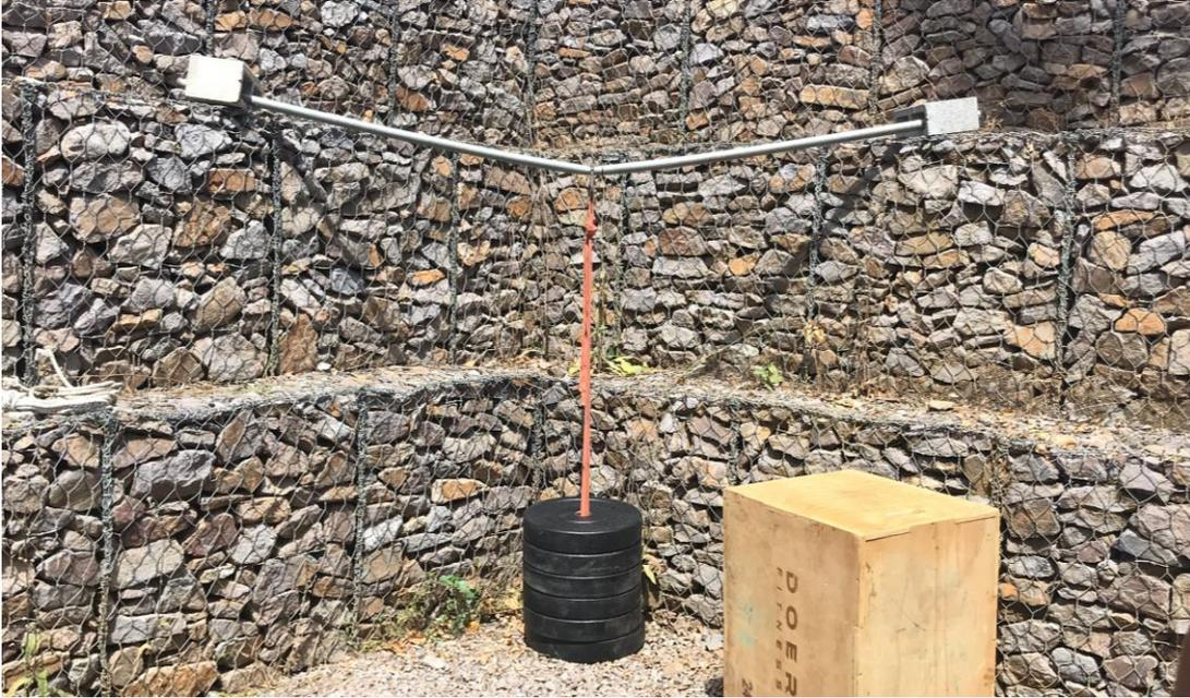
**Figure 18:** The bending point of our system occurred with a weight of 270 pounds.
