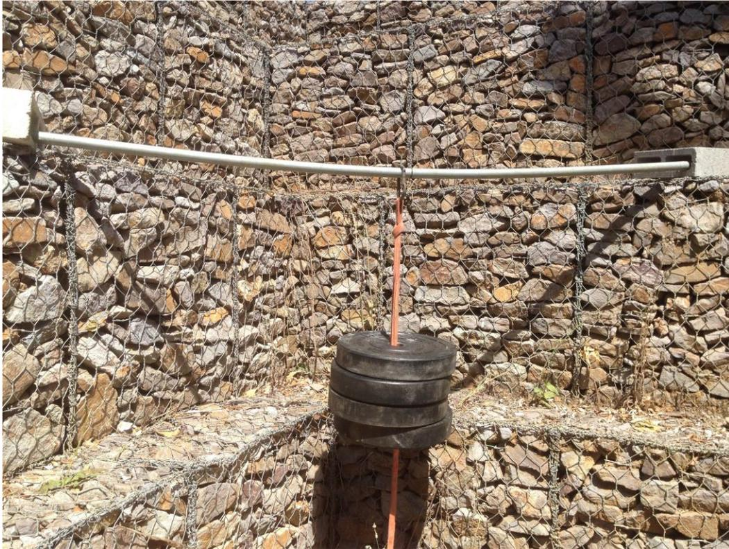
**Figure 17:** Slight deformation when 180 pound load applied to the weakest point of pole.
