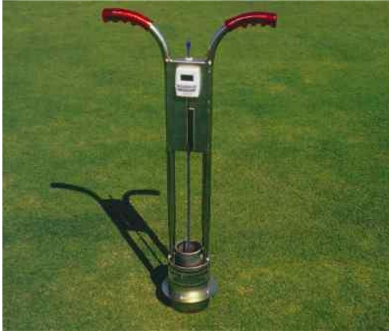
**Figure 29:** The Turf-tec Infiltration Measuring Device (IN2-W)
