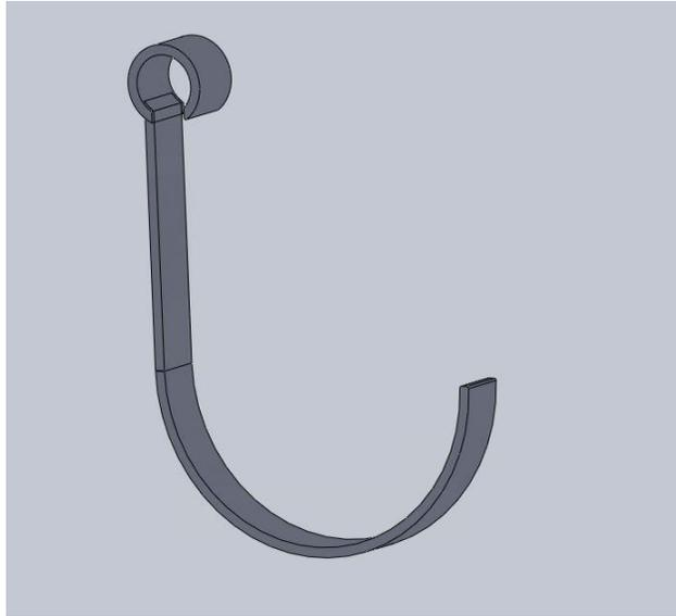
**Figure 23:** The Gutter Hook Attachment
