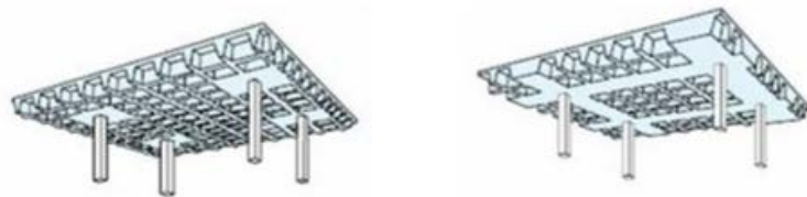
Figure 2: Waffle Slab with Solid Heads (left), Waffle Slab with Band Beams (right) 2
