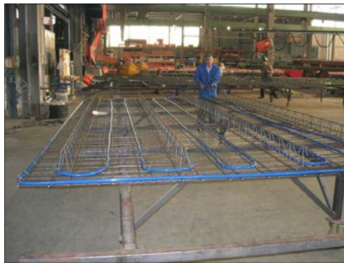
Figure 8: Radiant heating and cooling system implemented in the factory setting *courtesy of Bubbledeck North America
