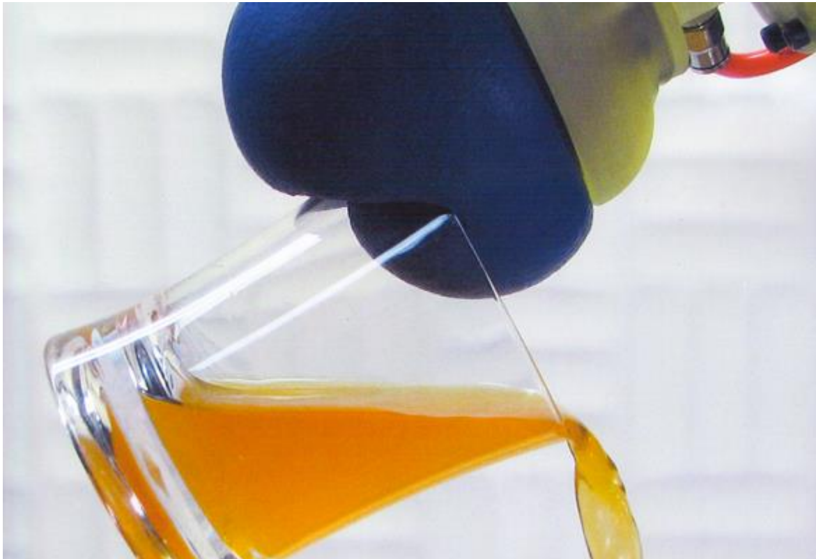
Figure 2-3 Universal Jamming Gripper picking up a glass of juice 8
