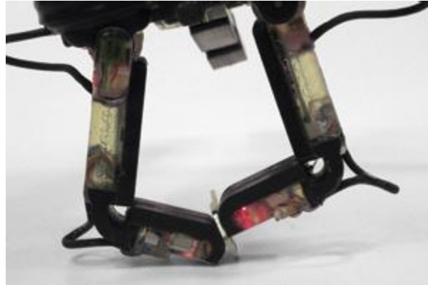
Figure 2-5 The same fingers would deform differently to grasp different objects 9
