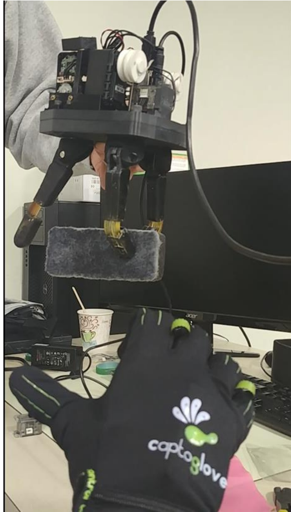
Figure 7-1: Human controlling the robotics hand to pick up a board eraser
