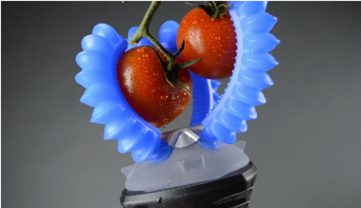
Figure 2-2 Soft Robotics Inc.'s gripper holding some tomatoes 7
