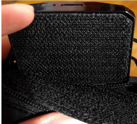
Figure 6-9 Provided Velcro surface beneath the CaptoGlove textile
