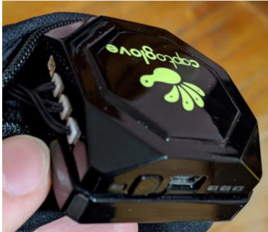
Figure 6-8 CaptoGlove housing with USB and sensor ports
