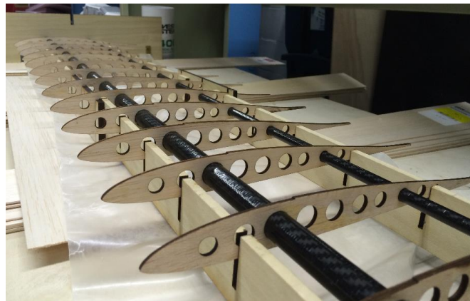
Figure 7.2 - Carbon Fiber Wing Spars
