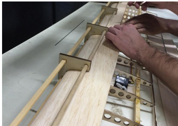
Figure 7.1 - Balsa Wood Ribs and Balsa Wood Leading Edge Wrap
