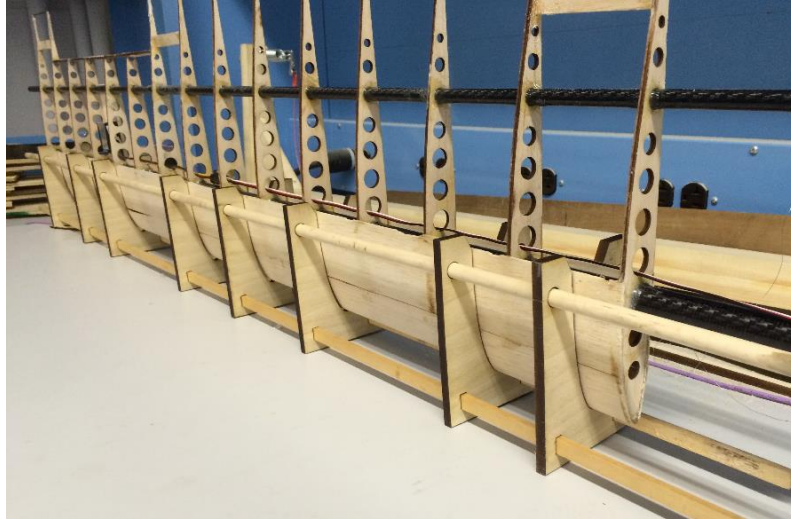
Figure 7.5 - Production Aircraft Wing Construction with Balsa Leading Edge Wrap and Laminated Balsa Plywood Ribs
