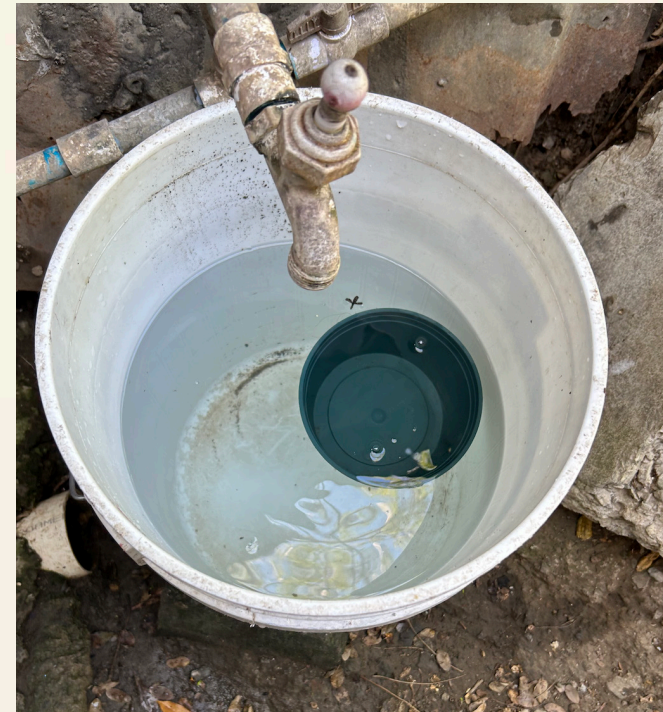
Figure 12: 5-gallon Holding Bucket in La Libertad showing visible sediment and bugs present in the water (tested positive for E.coli)
