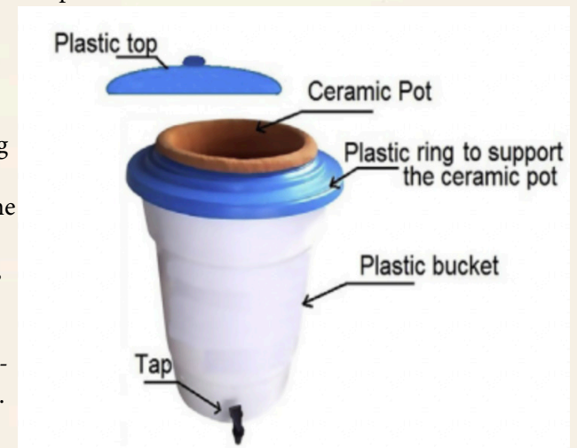
Figure 5: Ceramic Filtration Mechanism 25
