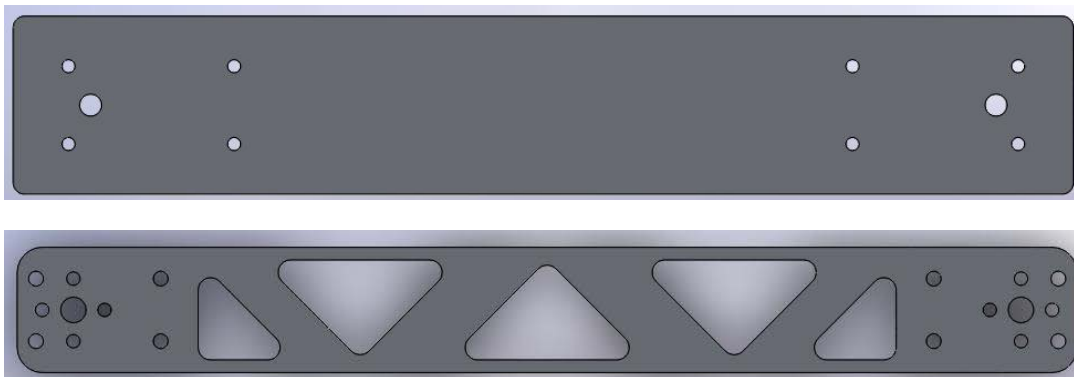
Figure 40: Comparison between the old Thigh Plate (Top) and the new Leg Plate (Bottom)
