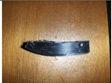
Figure 33 - Rubber Pad missing piece
