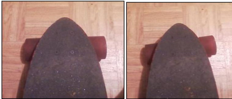
Figure 4 - Board with front wheels strait (left) and with wheels slightly turned (right)
